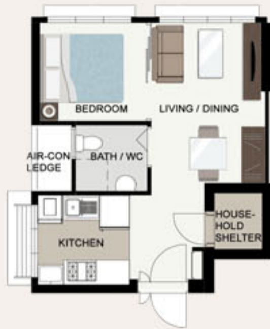
LAYOUT IDEAS FOR 2-ROOM (TYPE 1) APPROX. FLOOR AREA 38 sqm (Inclusive of Internal Floor Area of 36 sqm and Air-Con Ledge)
