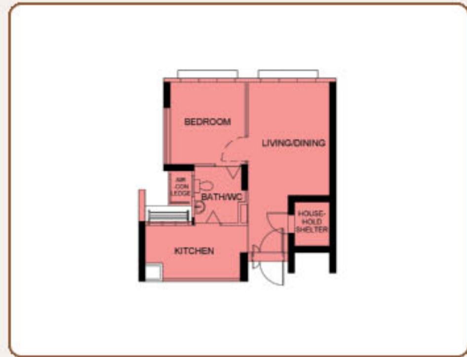
TYPICAL 2-ROOM (TYPE 2) FLOOR PLAN APPROX. FLOOR AREA 47 sqm (Inclusive of Internal Floor Area of 45 sqm and Air-Con Ledge)
