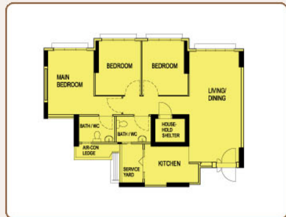
TYPICAL 4-ROOM FLOOR PLAN APPROX. FLOOR AREA 93 sqm (Inclusive of Internal Floor Area of 90 sqm and Air-Con Ledge)
