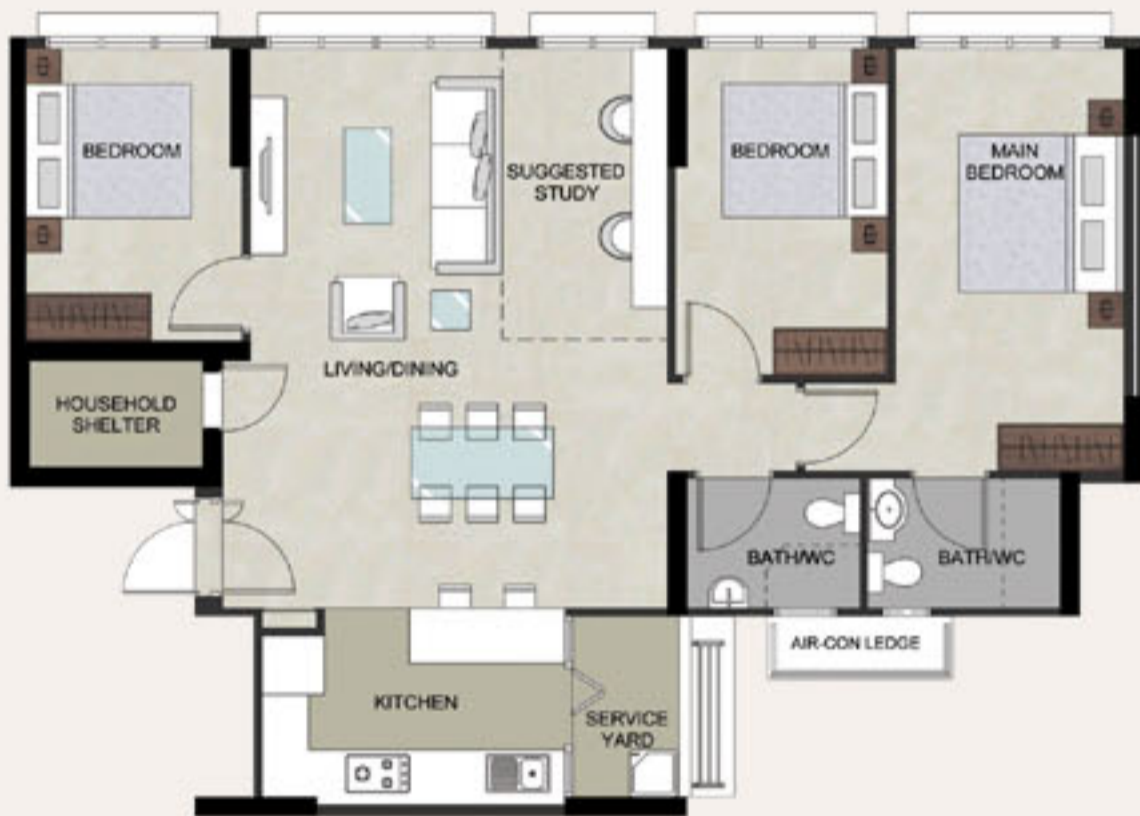
LAYOUT IDEAS FOR 5-ROOM APPROX. FLOOR AREA 112 sqm (Inclusive of Internal Floor Area of 110 sqm and Air-Con Ledge)
