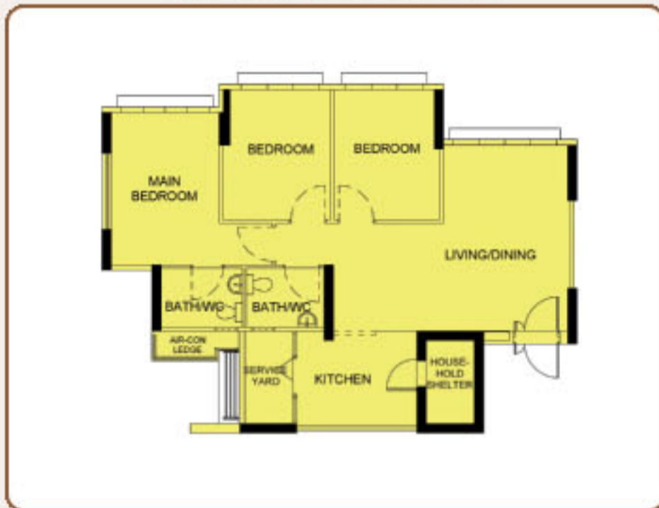
TYPICAL 4-ROOM FLOOR PLAN APPROX. FLOOR AREA 92 sqm (Inclusive of Internal Floor Area of 90 sqm and Air-Con Ledge)
