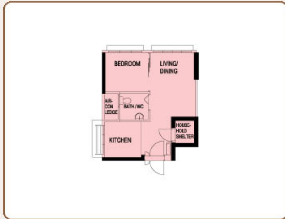
TYPICAL 2-ROOM (TYPE 1) FLOOR PLAN APPROX. FLOOR AREA 38 sqm (Inclusive of Internal Floor Area of 36 sqm and Air-Con Ledge)
