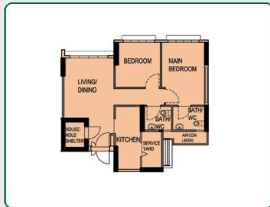
TYPICAL 3-ROOM FLOOR PLAN APPROX. FLOOR AREA 68 sqm (Inclusive of Internal Floor Area of 65 sqm and Air-Con Ledge)
