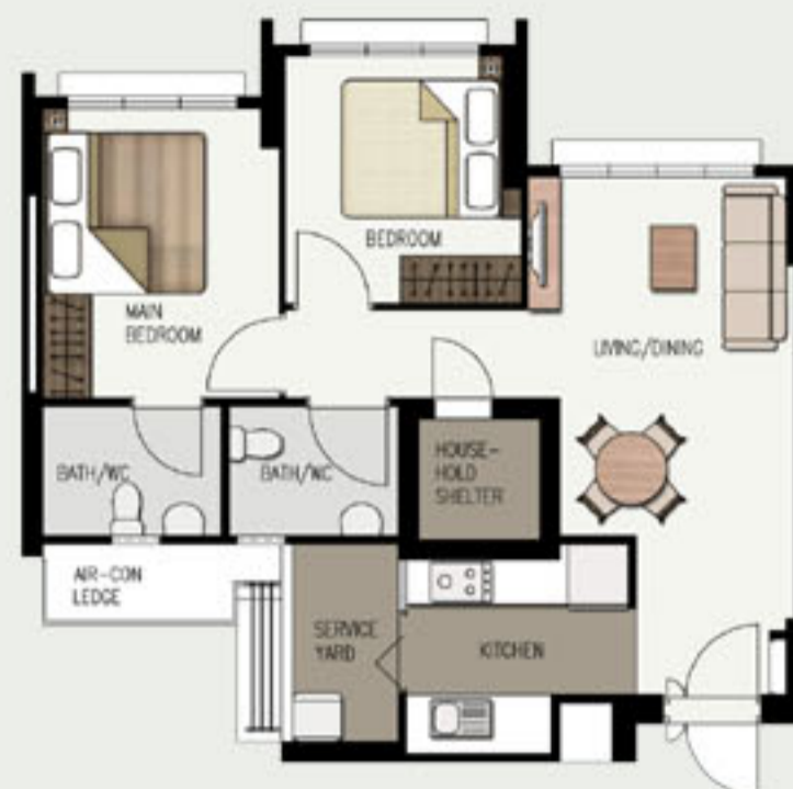
LAYOUT IDEAS FOR 3-ROOM APPROX. FLOOR AREA 68 sqm (Inclusive of Internal Floor Area 65 sqm and Air-Con Ledge)
