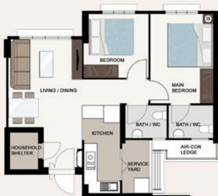
LAYOUT IDEAS FOR 3-ROOM APPROX. FLOOR AREA 68 sqm (Inclusive of Internal Floor Area 65 sqm and Air-Con Ledge)
