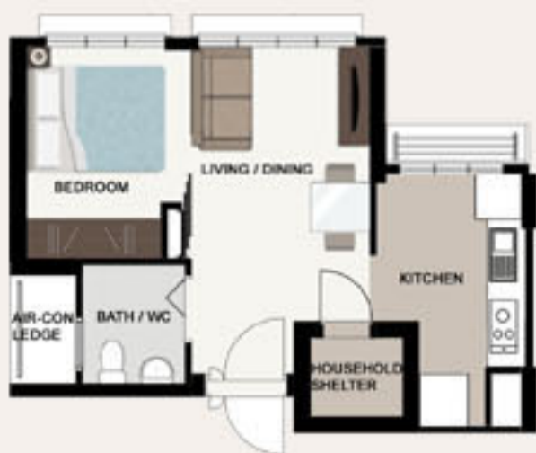
LAYOUT IDEAS FOR 2-ROOM (TYPE 1) APPROX. FLOOR AREA 38 sqm (Inclusive of Internal Floor Area of 36 sqm and Air-Con Ledge)
