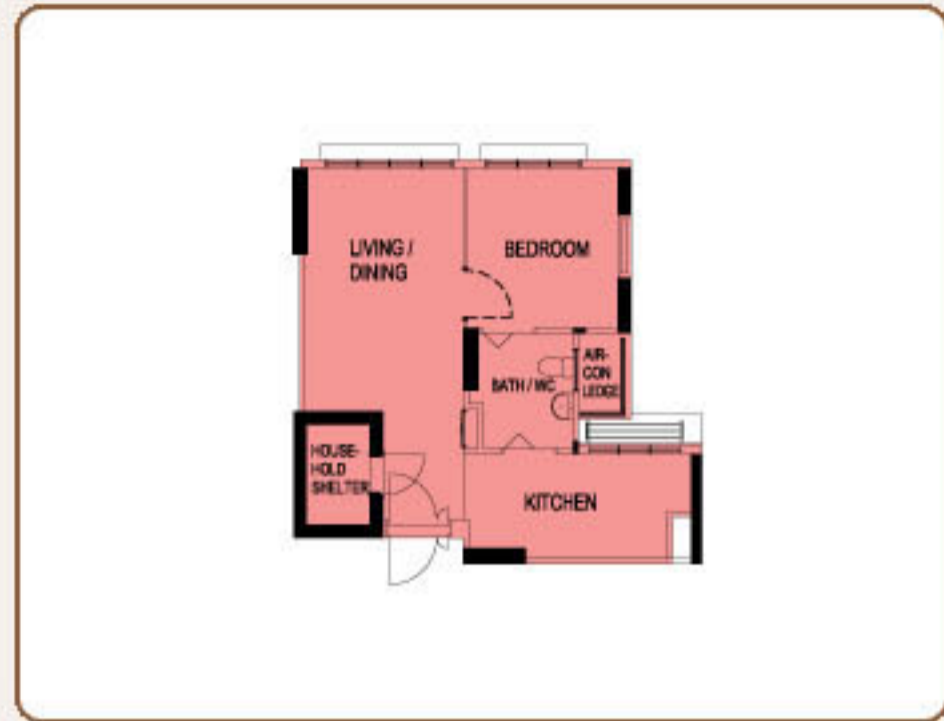
TYPICAL 2-ROOM (TYPE 2) FLOOR PLAN APPROX. FLOOR AREA 47 sqm (Inclusive of Internal Floor Area 45 sqm and Air-Con Ledge)
