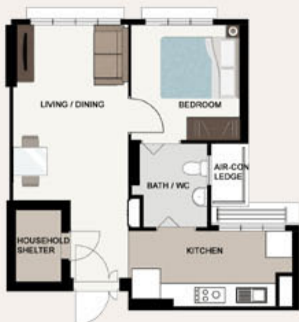
LAYOUT IDEAS FOR 2-ROOM (TYPE 2) APPROX. FLOOR AREA 47 sqm (Inclusive of Internal Floor Area of 45 sqm and Air-Con Ledge)
