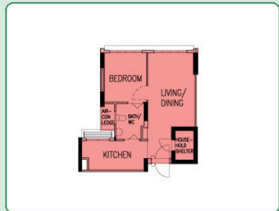
TYPICAL 2-ROOM (TYPE 2) FLOOR PLAN APPROX. FLOOR AREA 47 sqm (Inclusive of Internal Floor Area 45 sqm and Air-Con Ledge)
