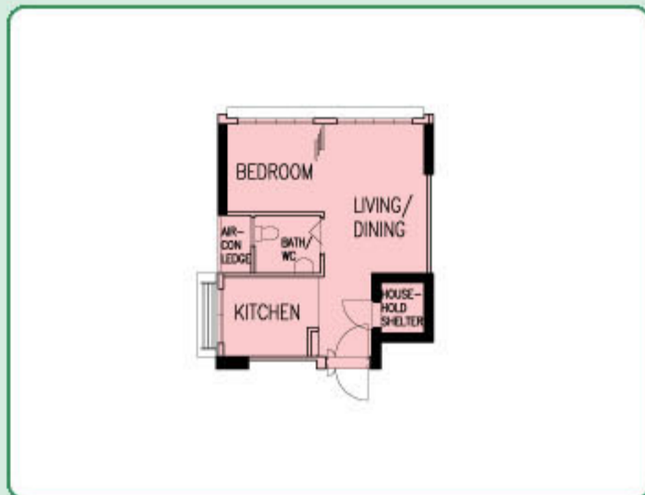
TYPICAL 2-ROOM (TYPE 1) FLOOR PLAN APPROX. FLOOR AREA 37 sqm (Inclusive of Internal Floor Area 35 sqm and Air-Con Ledge)
