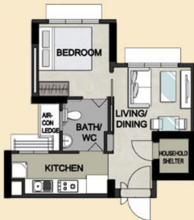
LAYOUT IDEAS FOR STUDIO APARTMENT (TYPE A) APPROX. FLOOR AREA 37 sqm (Inclusive of Internal Floor Area of 35 sqm and Air-Con Ledge)
