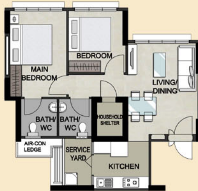
LAYOUT IDEAS FOR 3-ROOM APPROX. FLOOR AREA 67 sqm (Inclusive of Internal Floor Area 65 sqm and Air-Con Ledge)
