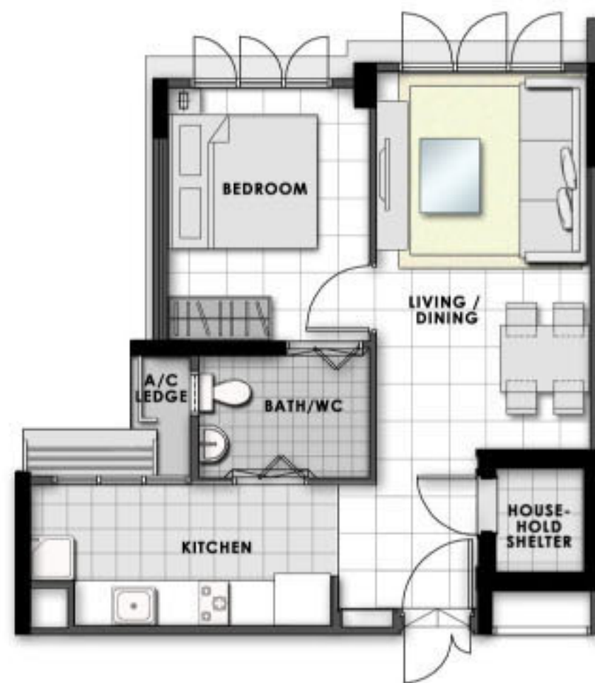
LAYOUT IDEAS FOR 2-ROOM APPROX. floor area 46 sqm (Inclusive of Internal Floor Area 45 sqm and Air-Con Ledge)
