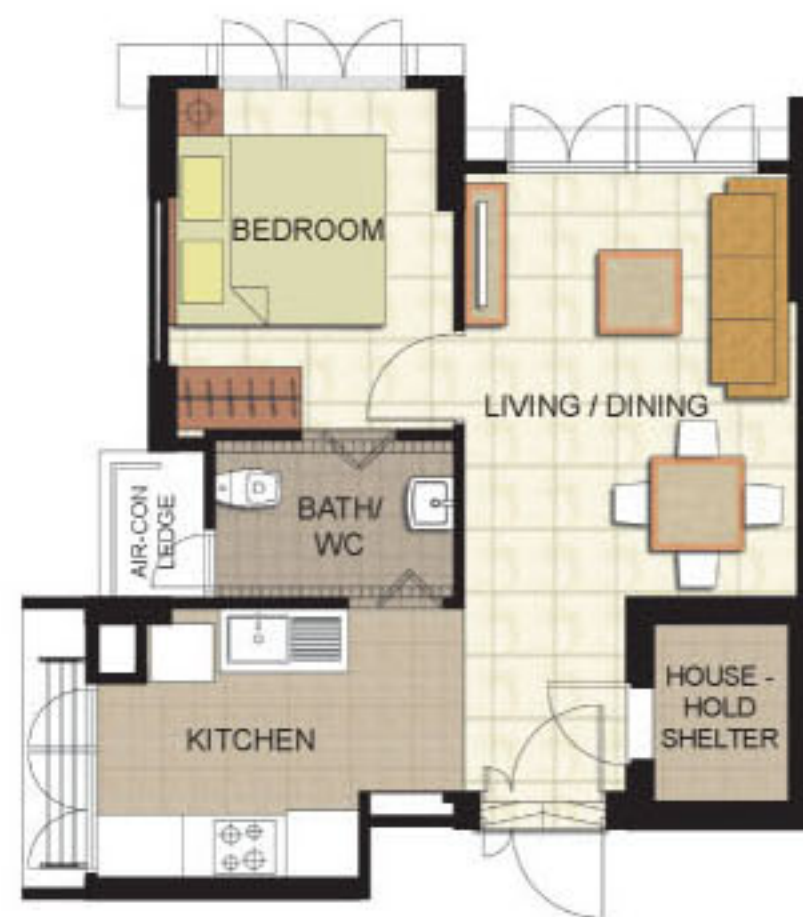
LAYOUT IDEAS FOR 2-ROOM APPROX. floor area 44 sqm (Inclusive of Internal Floor Area 42 sqm and Air-Con Ledge)
