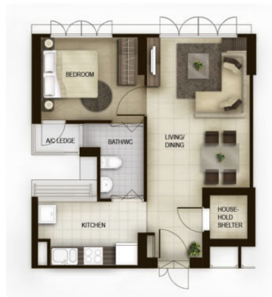
LAYOUT IDEAS FOR 2-ROOM APPROX. FLOOR AREA 47 sqm (Inclusive of Internal Floor Area 45 sqm and Air-Con Ledge)
