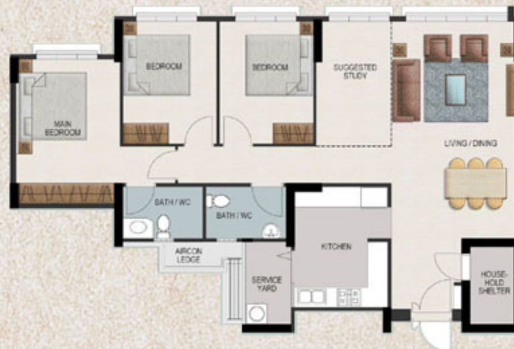
LAYOUT IDEAS FOR 5-ROOM (WITH SINGULAR KITCHEN) APPROX. FLOOR AREA 112 sqm (Inclusive of Internal Floor Area 110 sqm and Air-Con Ledge)
