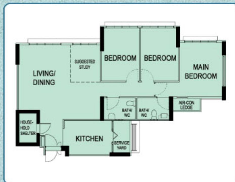
TYPICAL 5-ROOM FLOOR PLAN APPROX. FLOOR AREA 113 sqm (Inclusive of Internal Floor Area 110 sqm and Air-Con Ledge)
