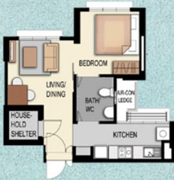
LAYOUT IDEAS FOR STUDIO APARTMENT (TYPE A) APPROX. FLOOR AREA 37 sqm (Inclusive of Internal Floor Area 35 sqm and Air-Con Ledge)
