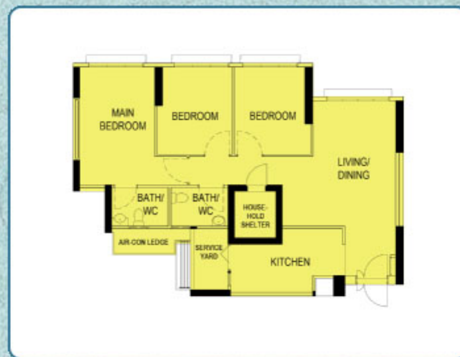
TYPICAL 4-ROOM FLOOR PLAN APPROX. FLOOR AREA 93 sqm (Inclusive of Internal Floor Area 90 sqm and Air-Con Ledge)
