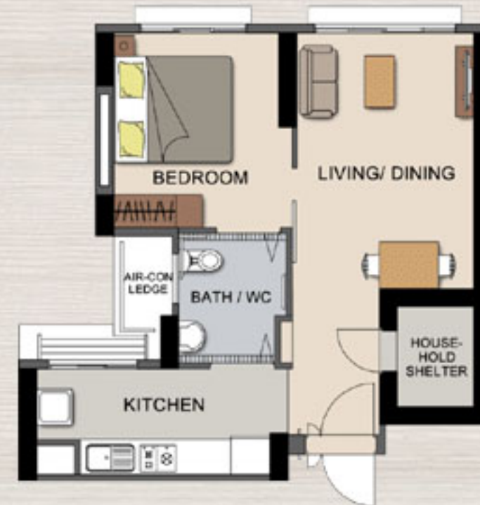
LAYOUT IDEAS FOR STUDIO APARTMENT (TYPE B) APPROX. FLOOR AREA 47 sqm (Inclusive of Internal Floor Area 45 sqm and Air-Con Ledge)
