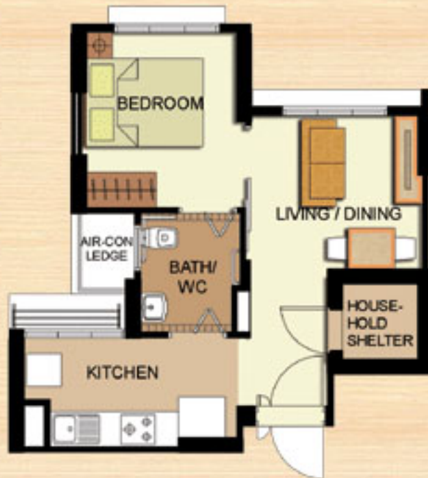
LAYOUT IDEAS FOR STUDIO APARTMENT (TYPE A) APPROX. FLOOR AREA 37 sqm (Inclusive of Internal Floor Area 35 sqm and Air-Con Ledge)
