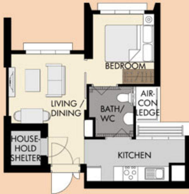
LAYOUT IDEAS FOR STUDIO APARTMENT (TYPE A) APPROX. FLOOR AREA 37 sqm (Inclusive of Internal Floor Area 35 sqm and Air-Con Ledge)
