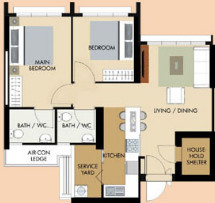
LAYOUT IDEAS FOR 3-ROOM APPROX. FLOOR AREA 68 sqm (Inclusive of Internal Floor Area 65 sqm and Air-Con Ledge)
