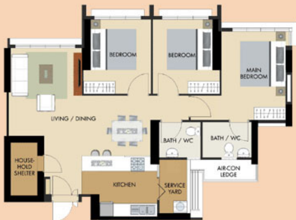
LAYOUT IDEAS FOR 4-ROOM APPROX. FLOOR AREA 93 sqm (Inclusive of Internal Floor Area 90 sqm and Air-Con Ledge)
