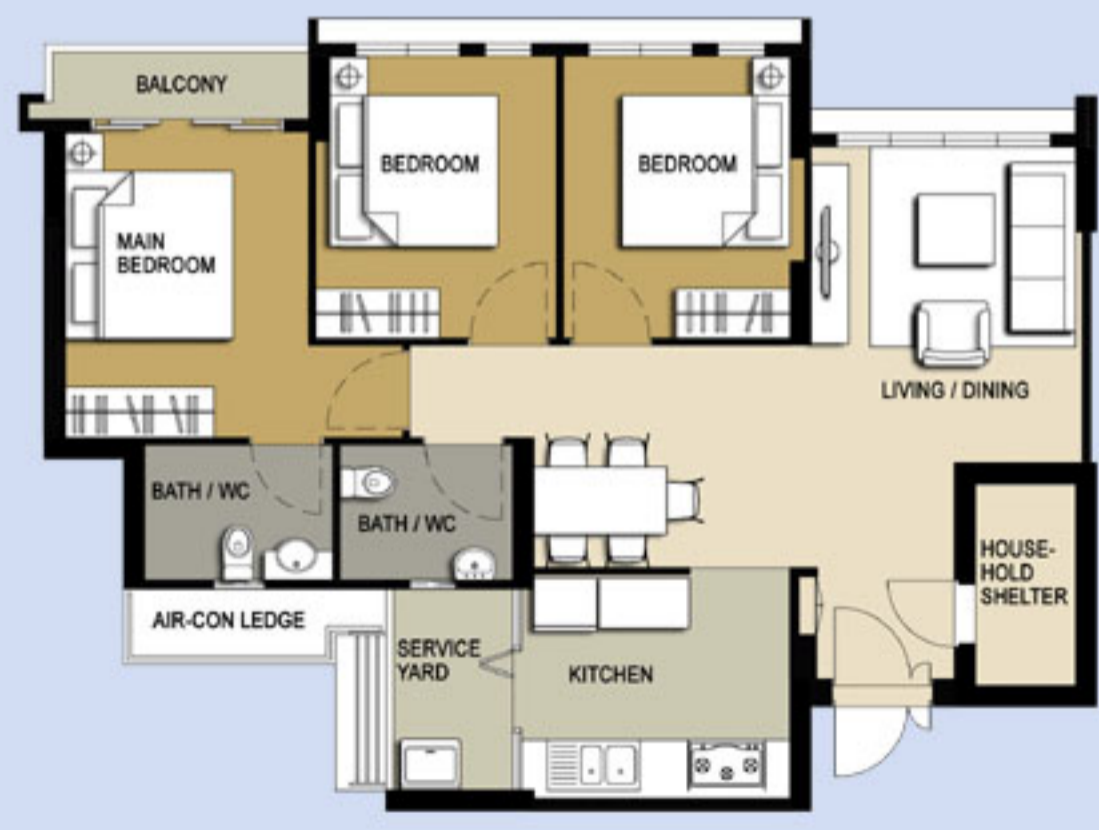
TYPICAL 4-ROOM FLOOR PLAN (WITH BALCONY) APPROX. FLOOR AREA 93 sqm (Inclusive of Internal Floor Area 90 sqm and Air-Con Ledge)
