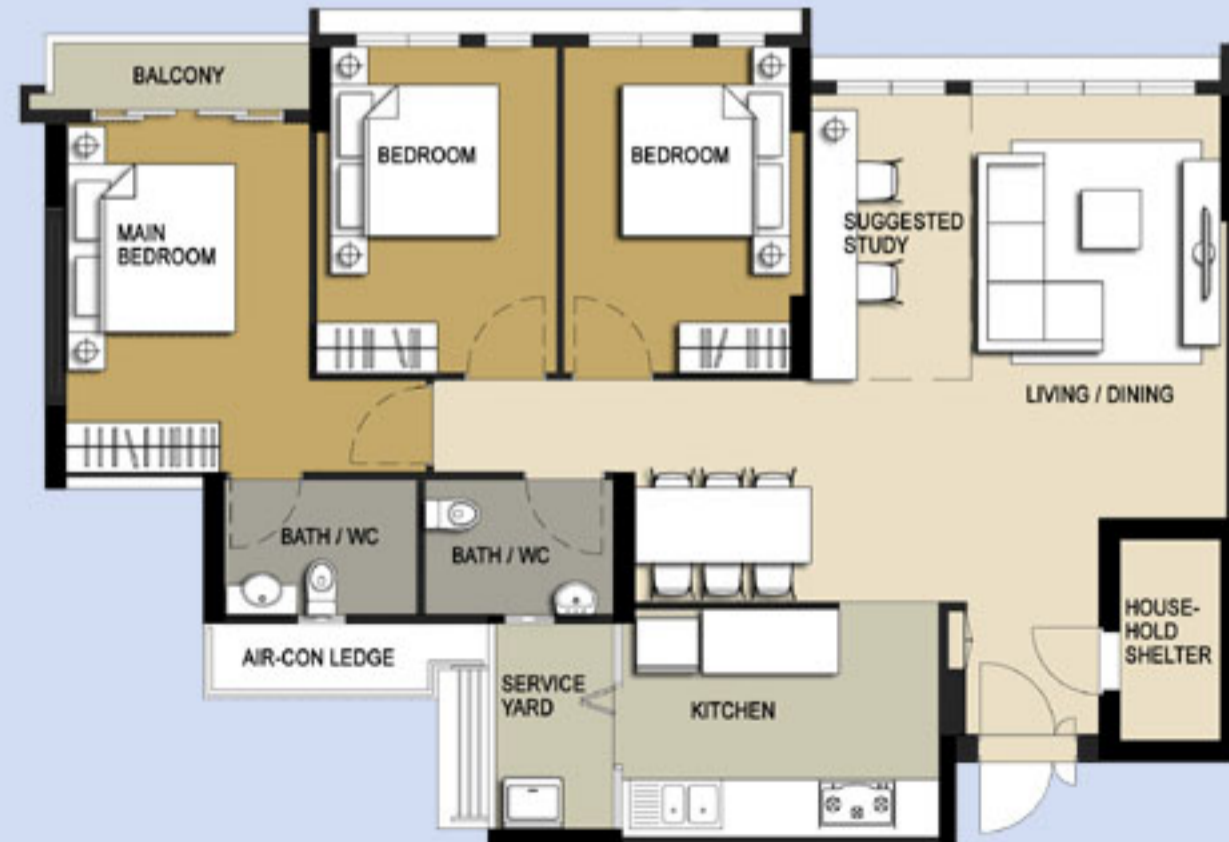
TYPICAL 5-ROOM FLOOR PLAN (WITH BALCONY) APPROX. FLOOR AREA 113 sqm (Inclusive of Internal Floor Area 110 sqm and Air-Con Ledge)
