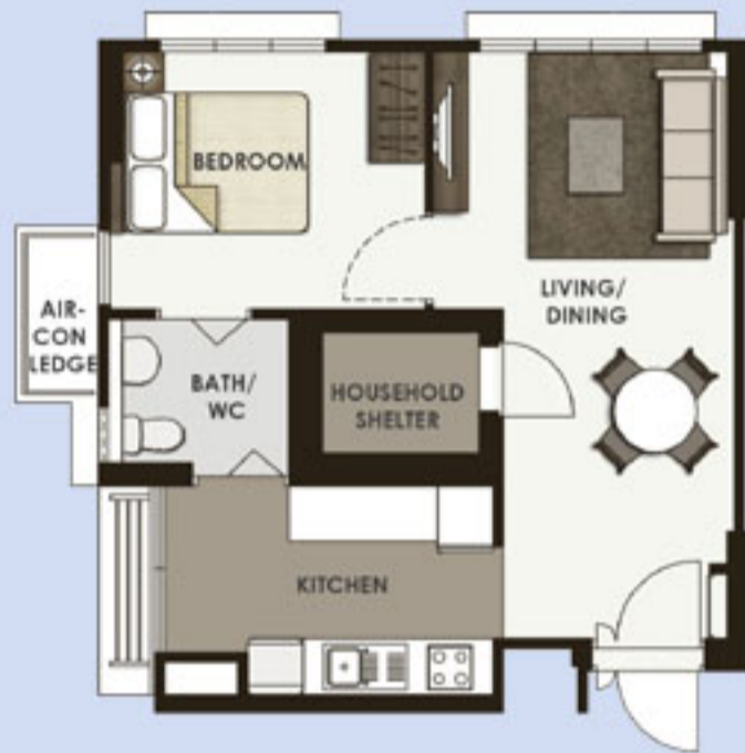
TYPICAL 2-ROOM FLOOR PLAN APPROX. FLOOR AREA 47 sqm (Inclusive of Internal Floor Area 45 sqm and Air-Con Ledge)
