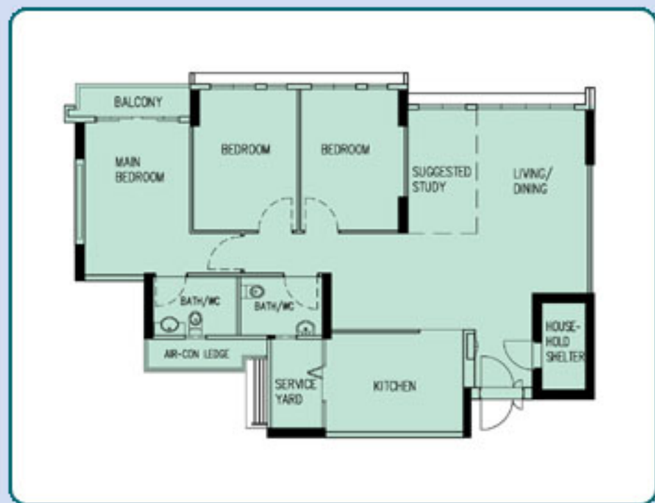
TYPICAL 5-ROOM FLOOR PLAN (WITH BALCONY) APPROX. FLOOR AREA 113 sqm (Inclusive of Internal Floor Area 110 sqm and Air-Con Ledge)
