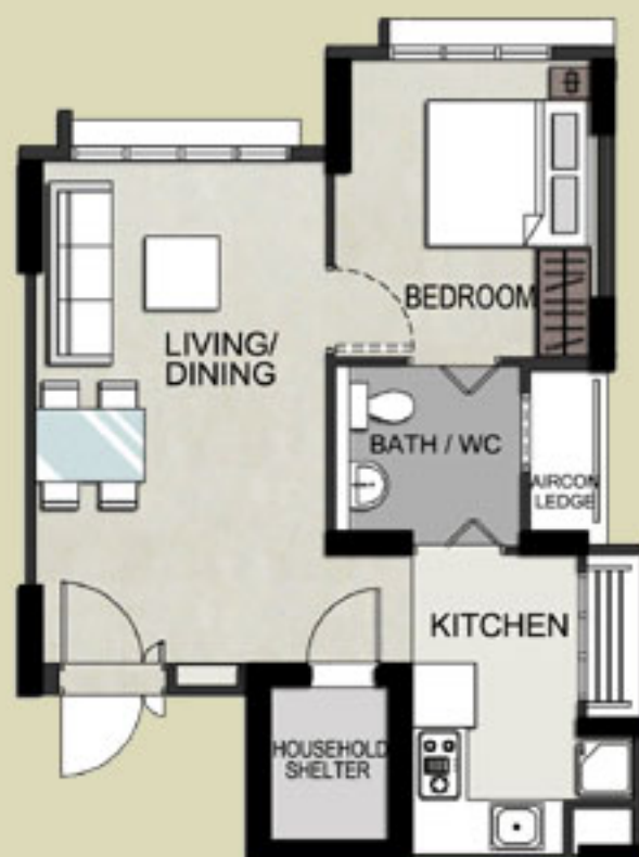
TYPICAL 2-ROOM FLOOR PLAN APPROX. FLOOR AREA 47 sqm (Inclusive of Internal Floor Area 45 sqm and Air-Con Ledge)
