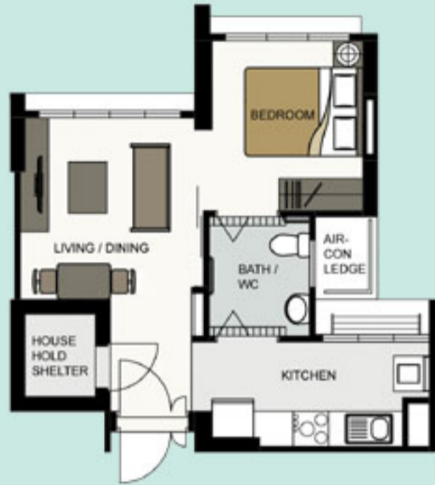
TYPICAL STUDIO APARTMENT (TYPE A) FLOOR PLAN APPROX. FLOOR AREA 37 sqm (Inclusive of Internal Floor Area 35 sqm and Air-Con Ledge)
