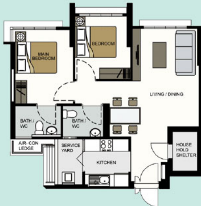
TYPICAL 3-ROOM FLOOR PLAN APPROX. FLOOR AREA 67 sqm (Inclusive of Internal Floor Area 65 sqm and Air-Con Ledge)
