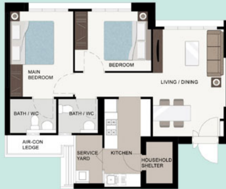
TYPICAL 3-ROOM FLOOR PLAN APPROX. FLOOR AREA 68 sqm (Inclusive of Internal Floor Area 65 sqm and Air-Con Ledge)
