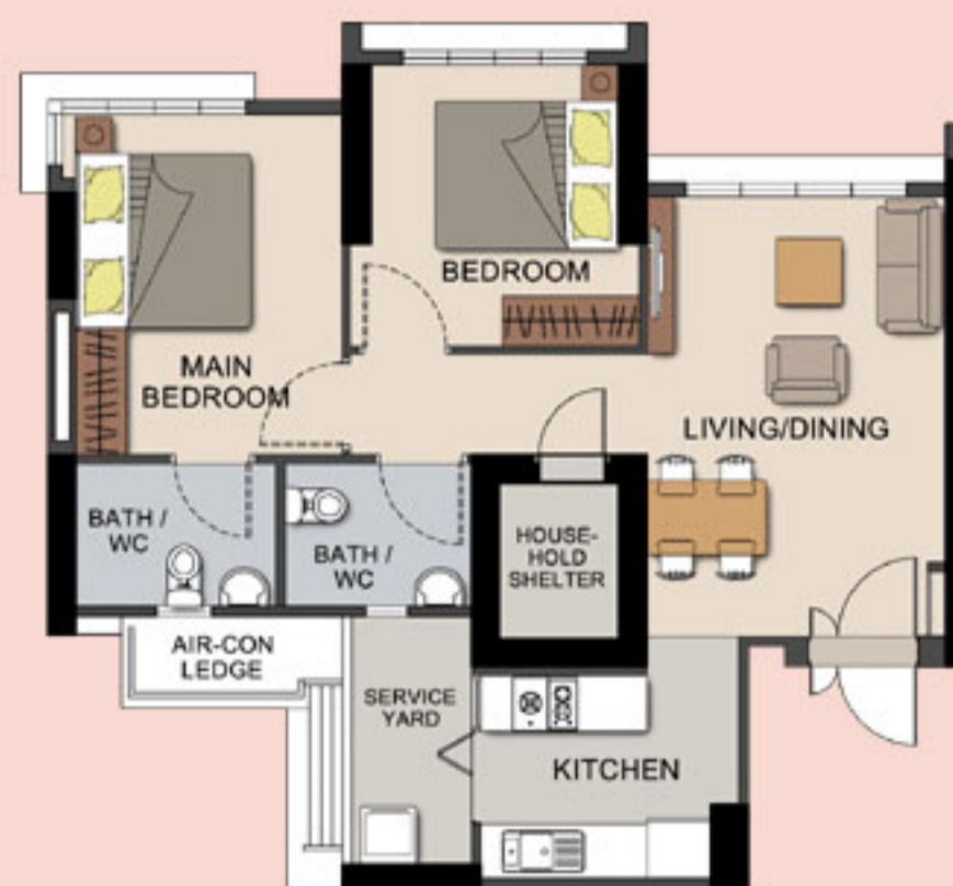
TYPICAL 3-ROOM FLOOR PLAN APPROX. FLOOR AREA 68 sqm (Inclusive of Internal Floor Area 65 sqm and Air-Con Ledge)
