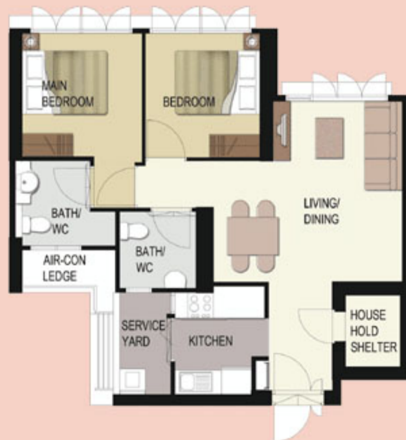
TYPICAL 3-ROOM FLOOR PLAN APPROX. FLOOR AREA 68 sqm (Inclusive of Internal Floor Area 65 sqm and Air-Con Ledge)
