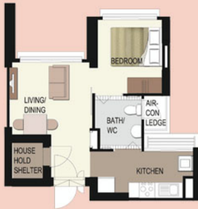
TYPICAL STUDIO APARTMENT (TYPE A) FLOOR PLAN APPROX. FLOOR AREA 37 sqm (Inclusive of Internal Floor Area 35 sqm and Air-Con Ledge)
