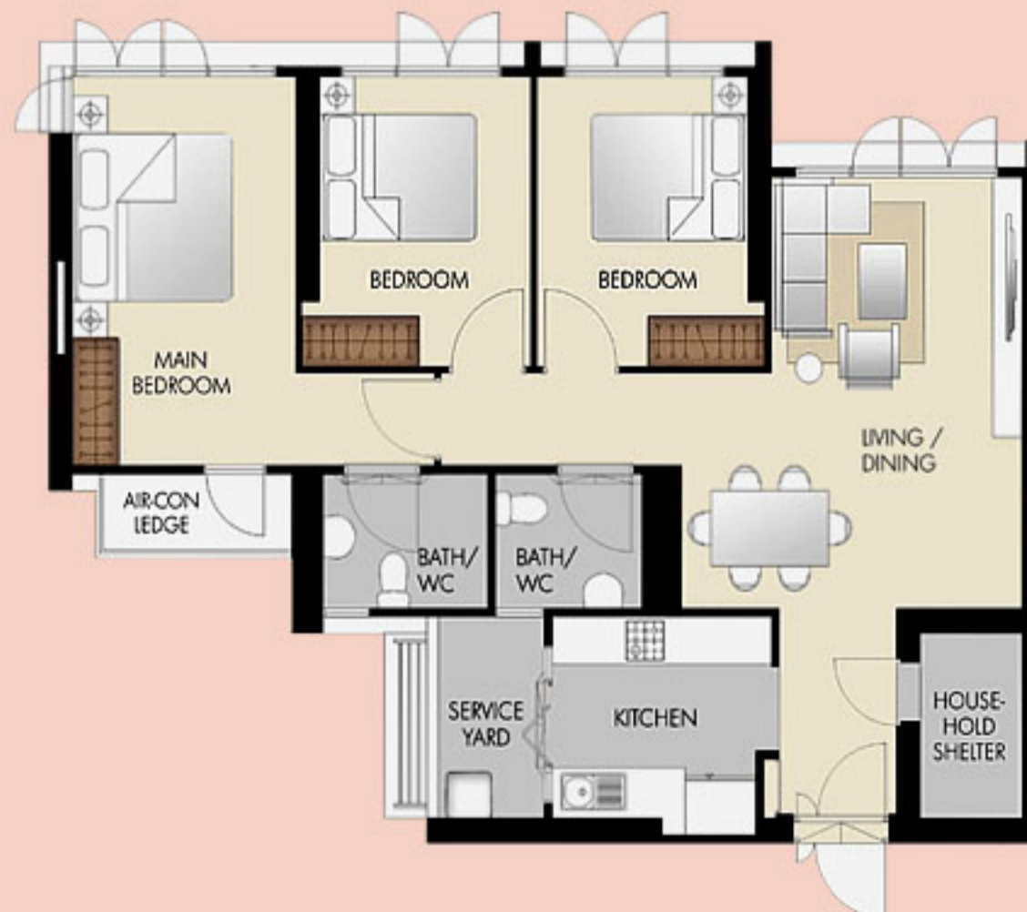
TYPICAL 4-ROOM FLOOR PLAN APPROX. FLOOR AREA 93 sqm (Inclusive of Internal Floor Area 90 sqm and Air-Con Ledge)
