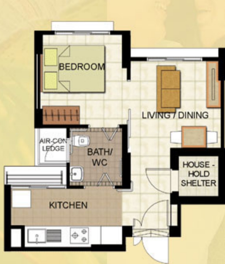
TYPICAL STUDIO APARTMENT (TYPE A) FLOOR PLAN APPROX. FLOOR AREA 37 sqm (Inclusive of Internal Floor Area 35 sqm and Air-Con Ledge)
