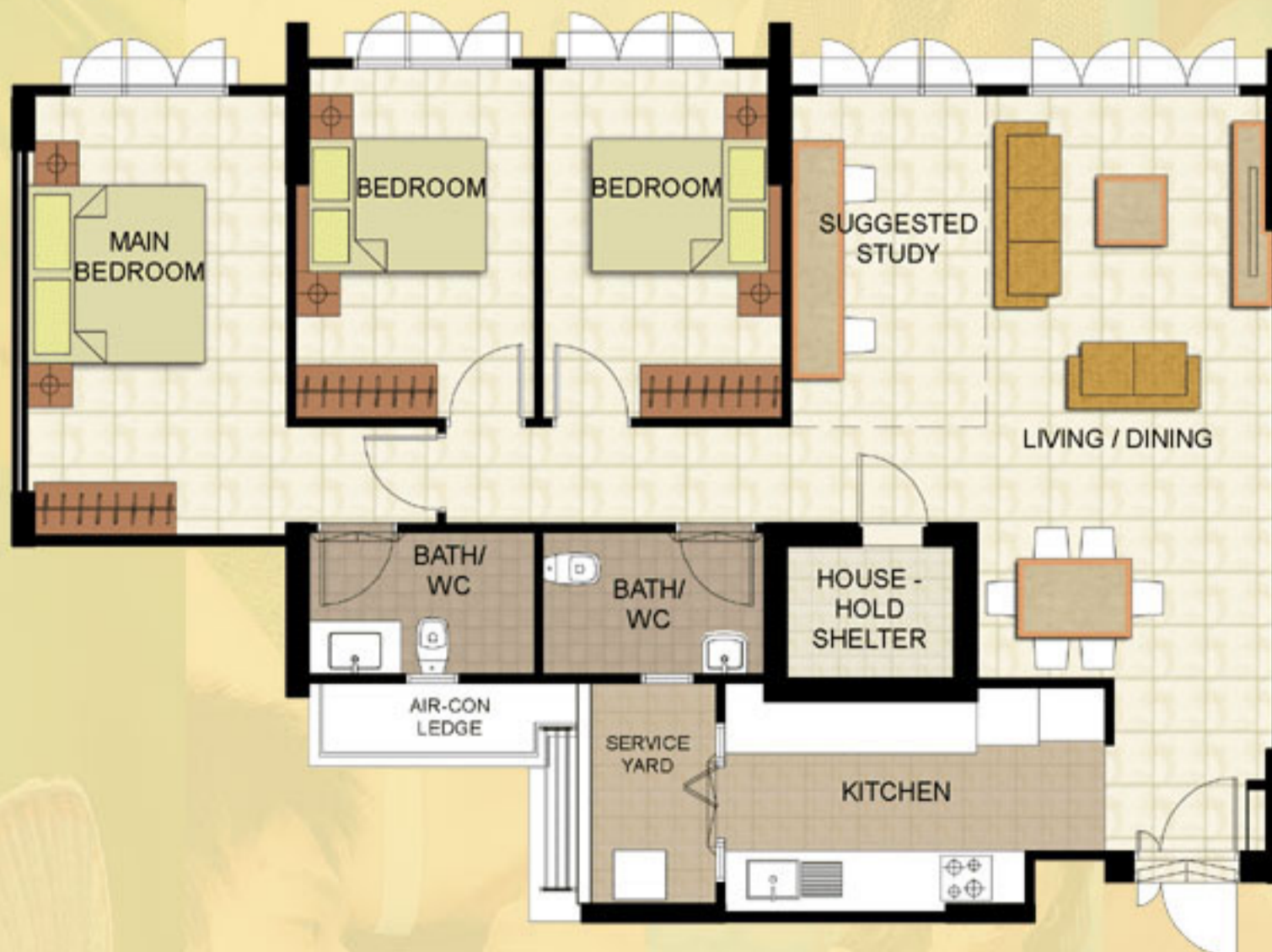
TYPICAL 5-ROOM FLOOR PLAN APPROX. FLOOR AREA 113 sqm (Inclusive of Internal Floor Area 110 sqm and Air-Con Ledge)
