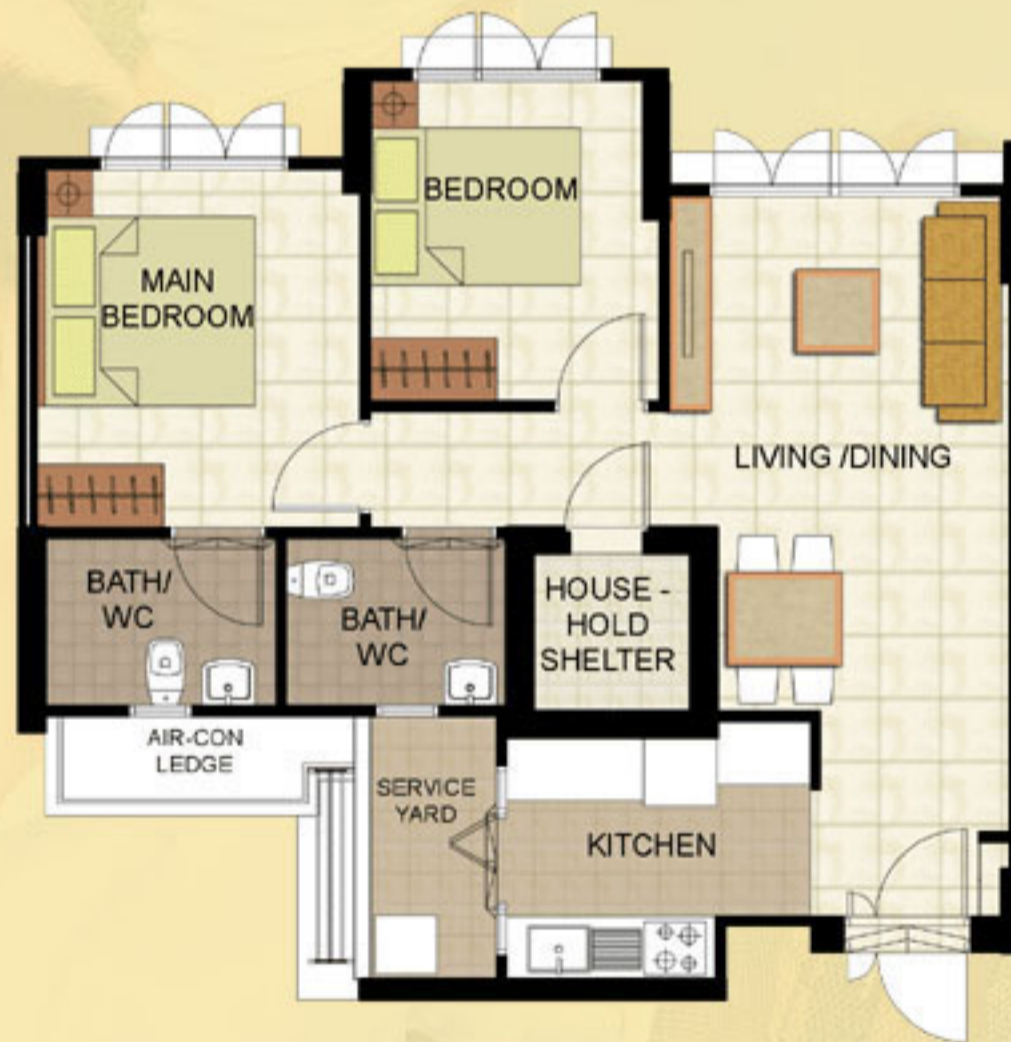
TYPICAL 3-ROOM FLOOR PLAN APPROX. FLOOR AREA 68 sqm (Inclusive of Internal Floor Area 65 sqm and Air-Con Ledge)
