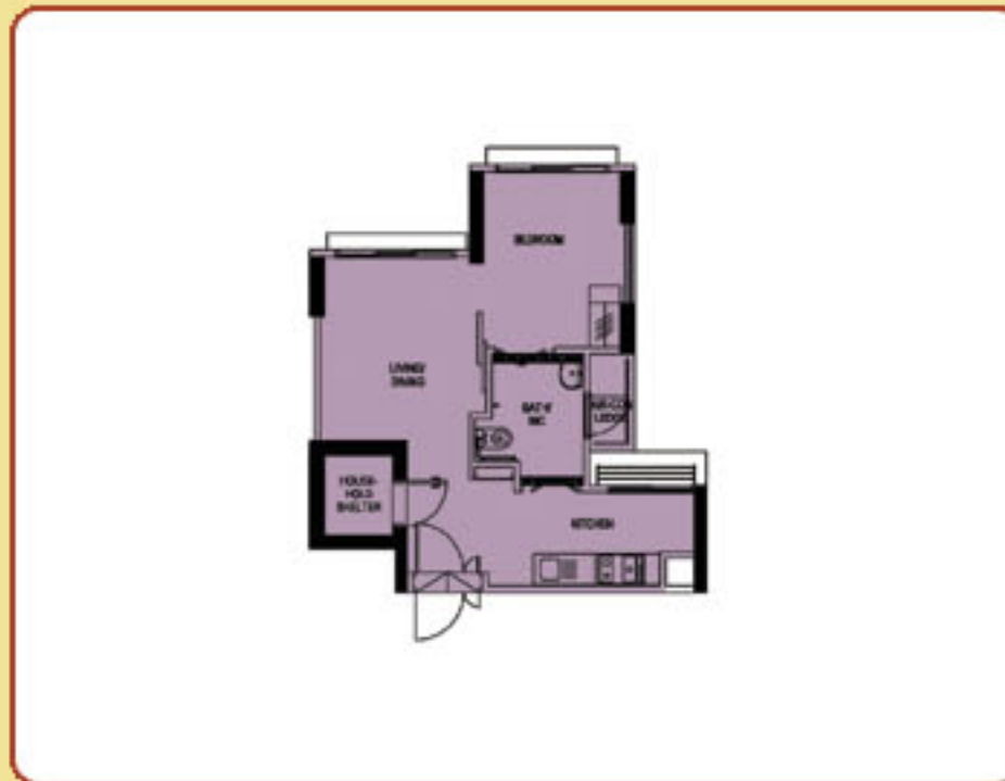
TYPICAL STUDIO APARTMENT (TYPE A) FLOOR PLAN APPROX. FLOOR AREA 36 sqm (Inclusive of Internal Floor Area 35 sqm and Air-Con Ledge)
