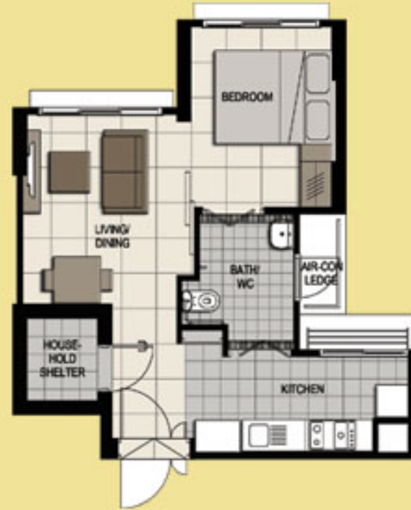
TYPICAL STUDIO APARTMENT (TYPE A) FLOOR PLAN APPROX. FLOOR AREA 36 sqm (Inclusive of Internal Floor Area 35 sqm and Air-Con Ledge)
