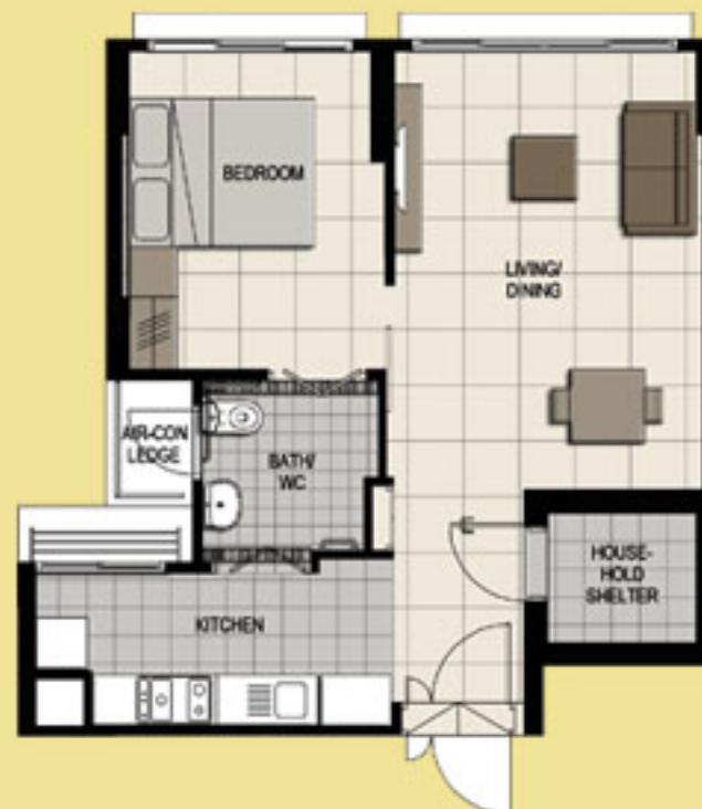
TYPICAL STUDIO APARTMENT (TYPE B) FLOOR PLAN APPROX. FLOOR AREA 46 sqm (Inclusive of Internal Floor Area 45 sqm and Air-Con Ledge)
