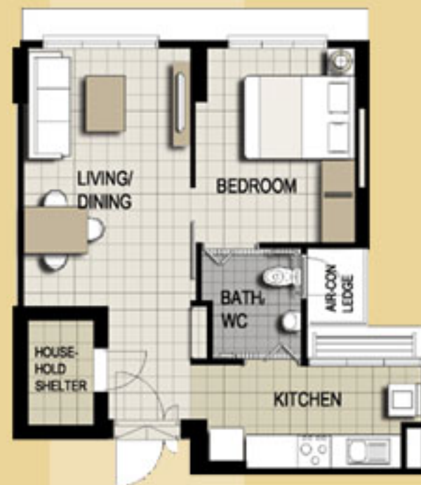
TYPICAL STUDIO APARTMENT (TYPE B) FLOOR PLAN APPROX. FLOOR AREA 47 sqm (Inclusive of Internal Floor Area 45 sqm and Air-Con Ledge)
