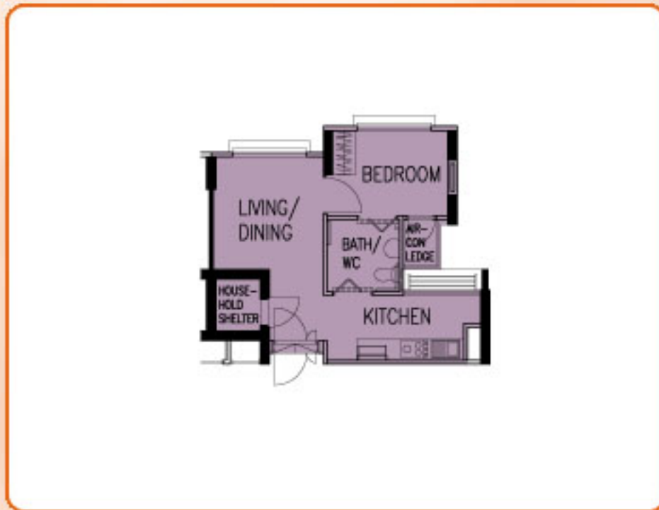
TYPICAL STUDIO APARTMENT (TYPE A) FLOOR PLAN APPROX. FLOOR AREA 37 sqm (Inclusive of Internal Floor Area 35 sqm and Air-Con Ledge)
