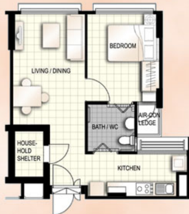
TYPICAL STUDIO APARTMENT (TYPE B) FLOOR PLAN APPROX. FLOOR AREA 47 sqm (Inclusive of Internal Floor Area 45 sqm and Air-Con Ledge)
