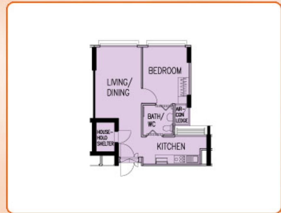
TYPICAL STUDIO APARTMENT (TYPE B) FLOOR PLAN APPROX. FLOOR AREA 47 sqm (Inclusive of Internal Floor Area 45 sqm and Air-Con Ledge)
