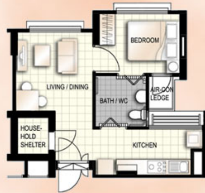
TYPICAL STUDIO APARTMENT (TYPE A) FLOOR PLAN APPROX. FLOOR AREA 37 sqm (Inclusive of Internal Floor Area 35 sqm and Air-Con Ledge)
