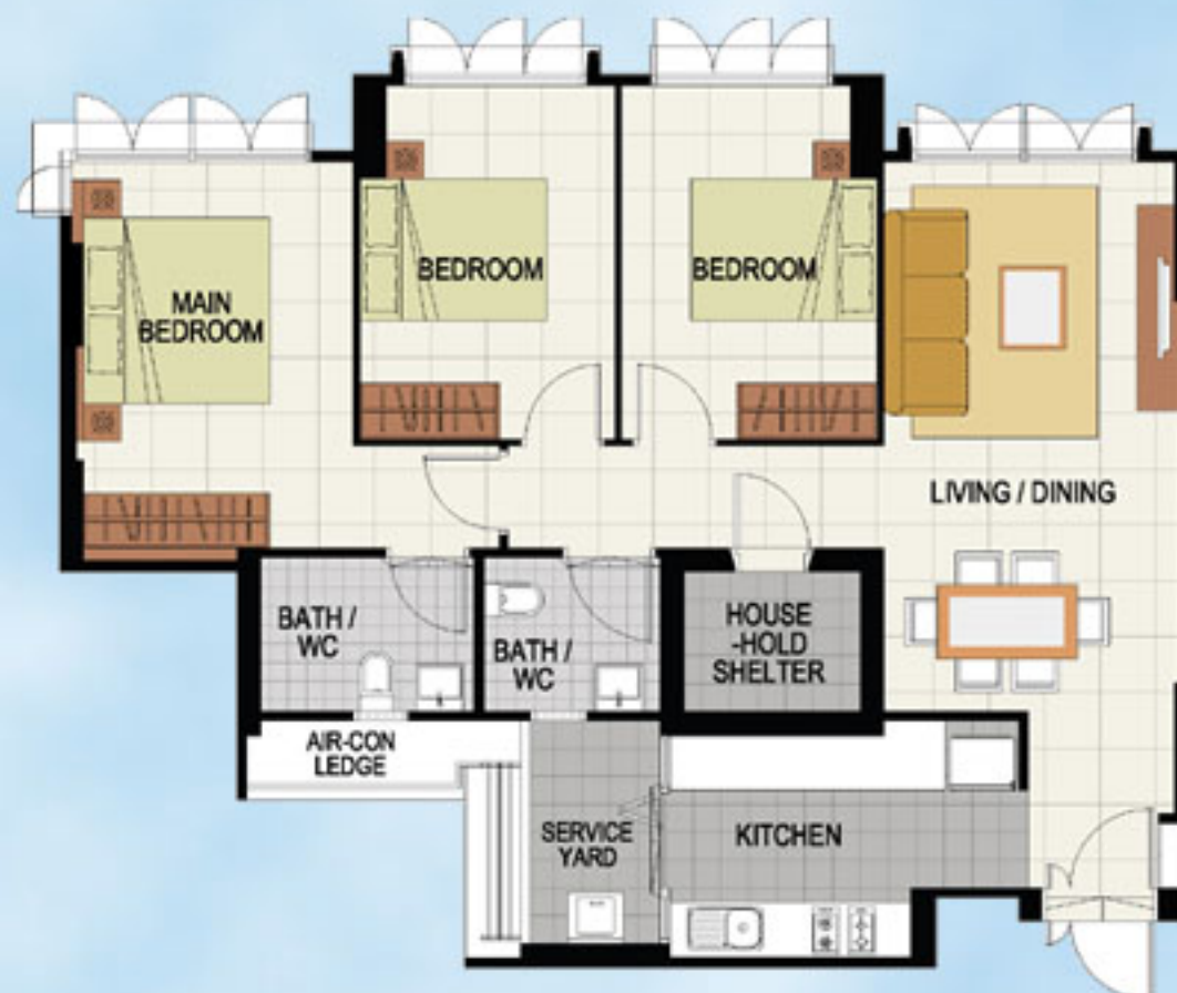
TYPICAL 4-ROOM FLOOR PLAN APPROX. FLOOR AREA 93 sqm (Inclusive of Internal Floor Area 90 sqm and Air-Con Ledge)
