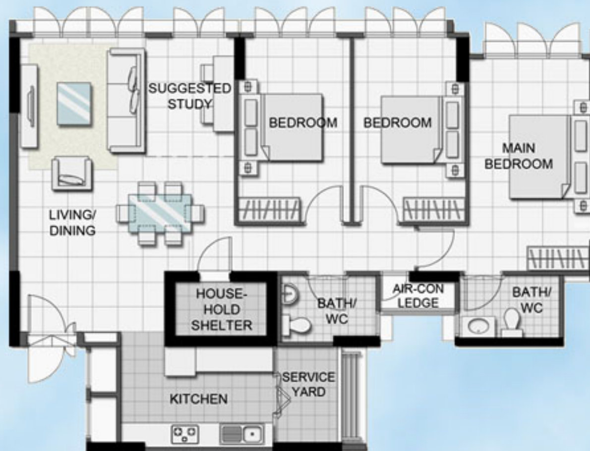
TYPICAL 5-ROOM FLOOR PLAN APPROX. FLOOR AREA 112 sqm (Inclusive of Internal Floor Area 110 sqm and Air-Con Ledge)
