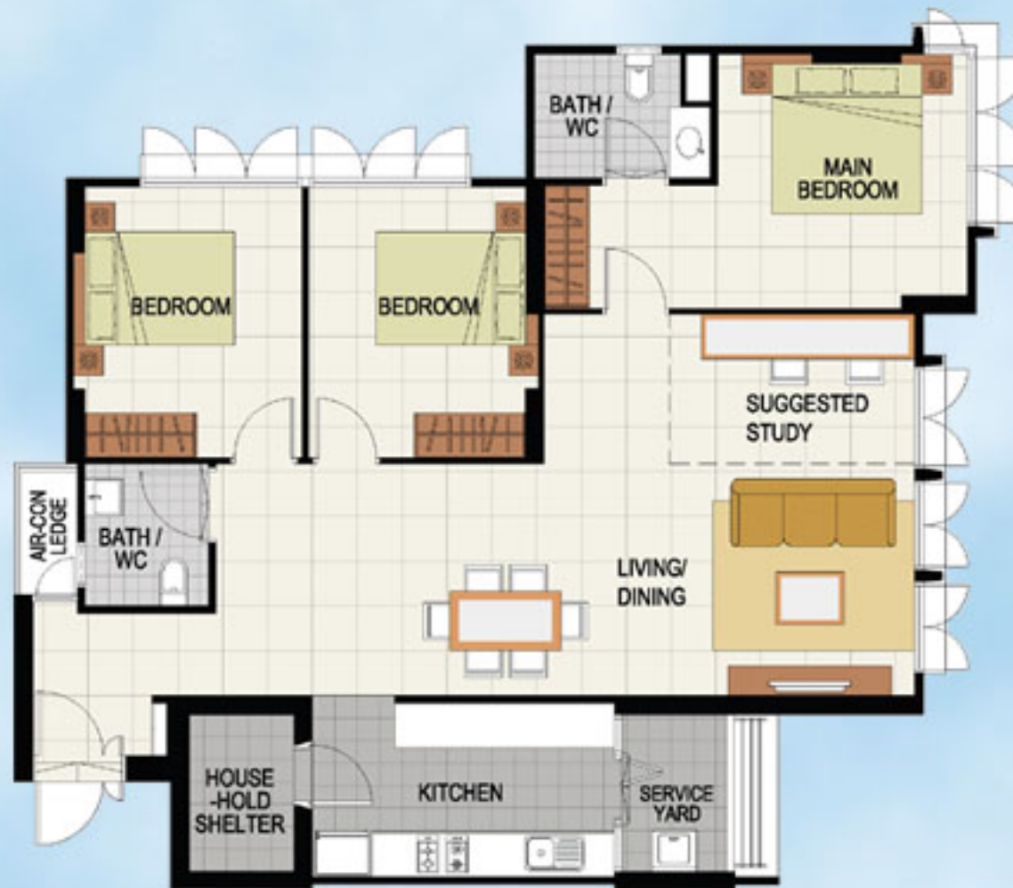
TYPICAL 5-ROOM FLOOR PLAN APPROX. FLOOR AREA 112 sqm (Inclusive of Internal Floor Area 110 sqm and Air-Con Ledge)
