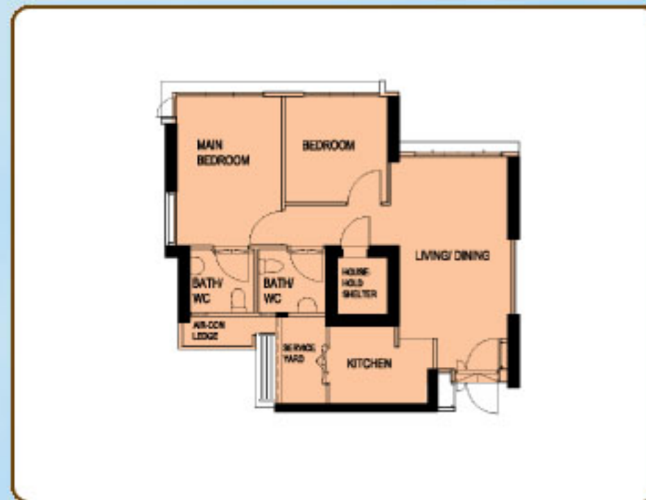
TYPICAL 3-ROOM FLOOR PLAN APPROX. FLOOR AREA 67 sqm (Inclusive of Internal Floor Area 65 sqm and Air-Con Ledge)
