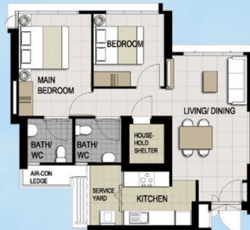
TYPICAL 3-ROOM FLOOR PLAN APPROX. FLOOR AREA 67 sqm (Inclusive of Internal Floor Area 65 sqm and Air-Con Ledge)
