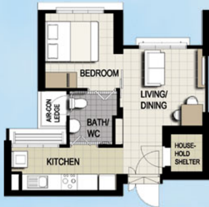
TYPICAL STUDIO APARTMENT (TYPE A) FLOOR PLAN APPROX. FLOOR AREA 37 sqm (Inclusive of Internal Floor Area 35 sqm and Air-Con Ledge)
