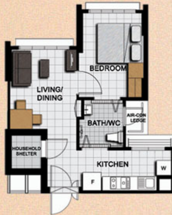
TYPICAL STUDIO APARTMENT (TYPE A) FLOOR PLAN APPROX. FLOOR AREA 37 sqm (Inclusive of Internal Floor Area 35 sqm and Air-Con Ledge)
