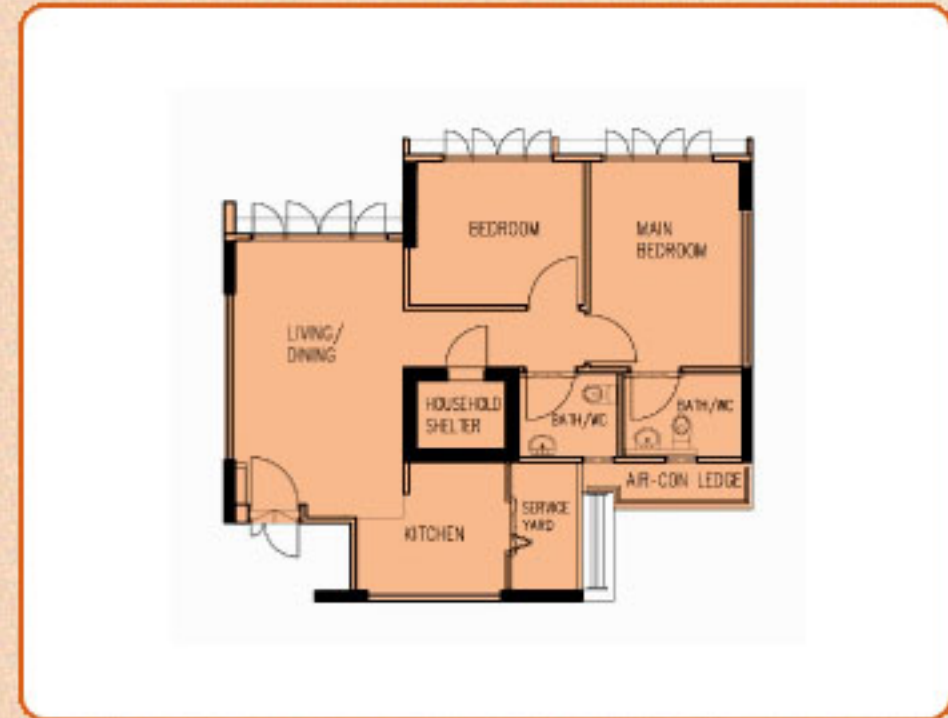
TYPICAL 3-ROOM FLOOR PLAN APPROX. FLOOR AREA 68 sqm (Inclusive of Internal Floor Area 65 sqm and Air-Con Ledge)
