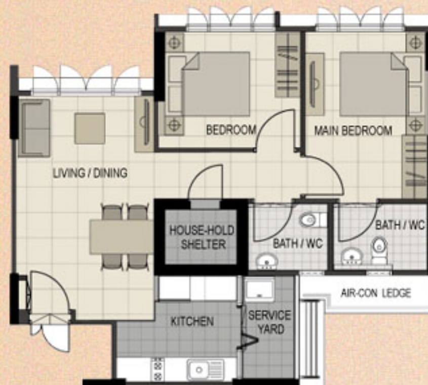
TYPICAL 3-ROOM FLOOR PLAN APPROX. FLOOR AREA 68 sqm (Inclusive of Internal Floor Area 65 sqm and Air-Con Ledge)
