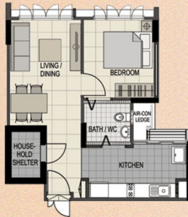
TYPICAL 2-ROOM FLOOR PLAN APPROX. FLOOR AREA 47 sqm (Inclusive of Internal Floor Area 45 sqm and Air-Con Ledge)
