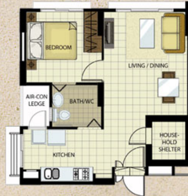
TYPICAL STUDIO APARTMENT FLOOR PLAN (TYPE B) APPROX. FLOOR AREA 47 sqm (Inclusive of Internal Floor Area 45 sqm and Air-Con Ledge)
