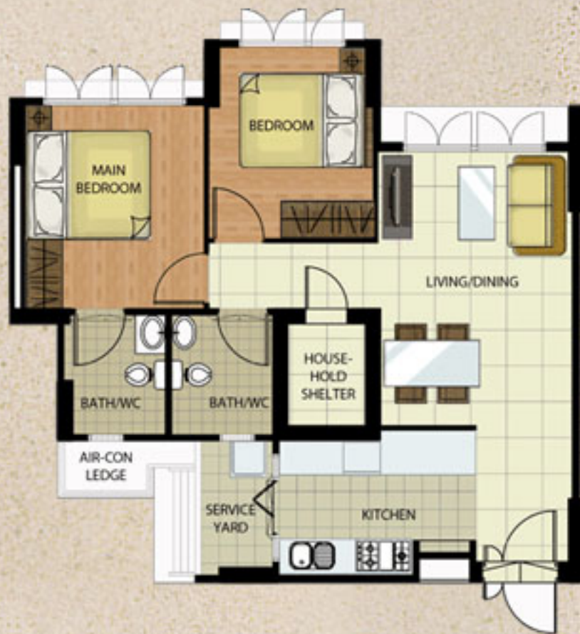
TYPICAL 3-ROOM FLOOR PLAN APPROX. FLOOR AREA 67 sqm (Inclusive of Internal Floor Area 65 sqm and Air-Con Ledge)
