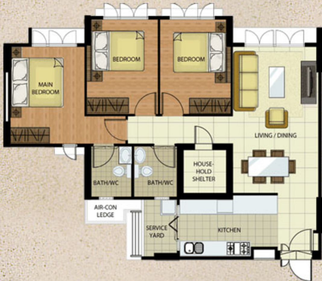
TYPICAL 4-ROOM FLOOR PLAN APPROX. FLOOR AREA 92 sqm (Inclusive of Internal Floor Area 90 sqm and Air-Con Ledge)
