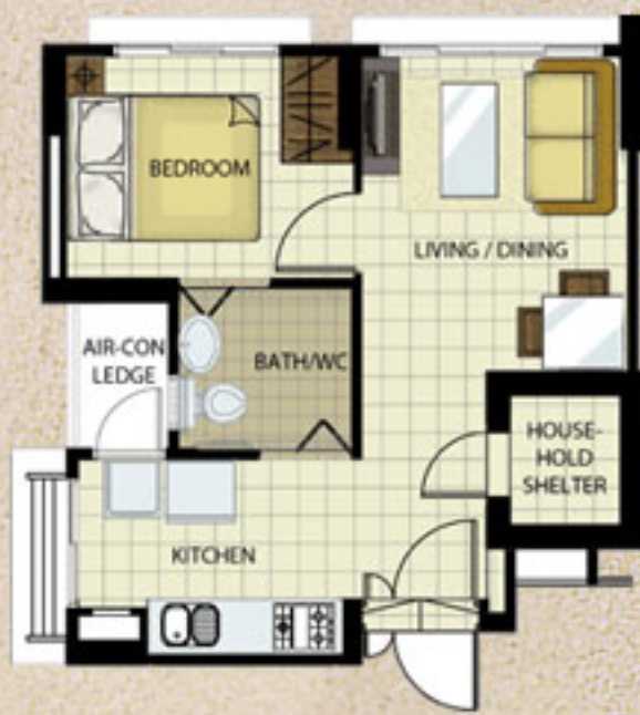
TYPICAL STUDIO APARTMENT FLOOR PLAN (TYPE A) APPROX. FLOOR AREA 37 sqm (Inclusive of Internal Floor Area 35 sqm and Air-Con Ledge)
