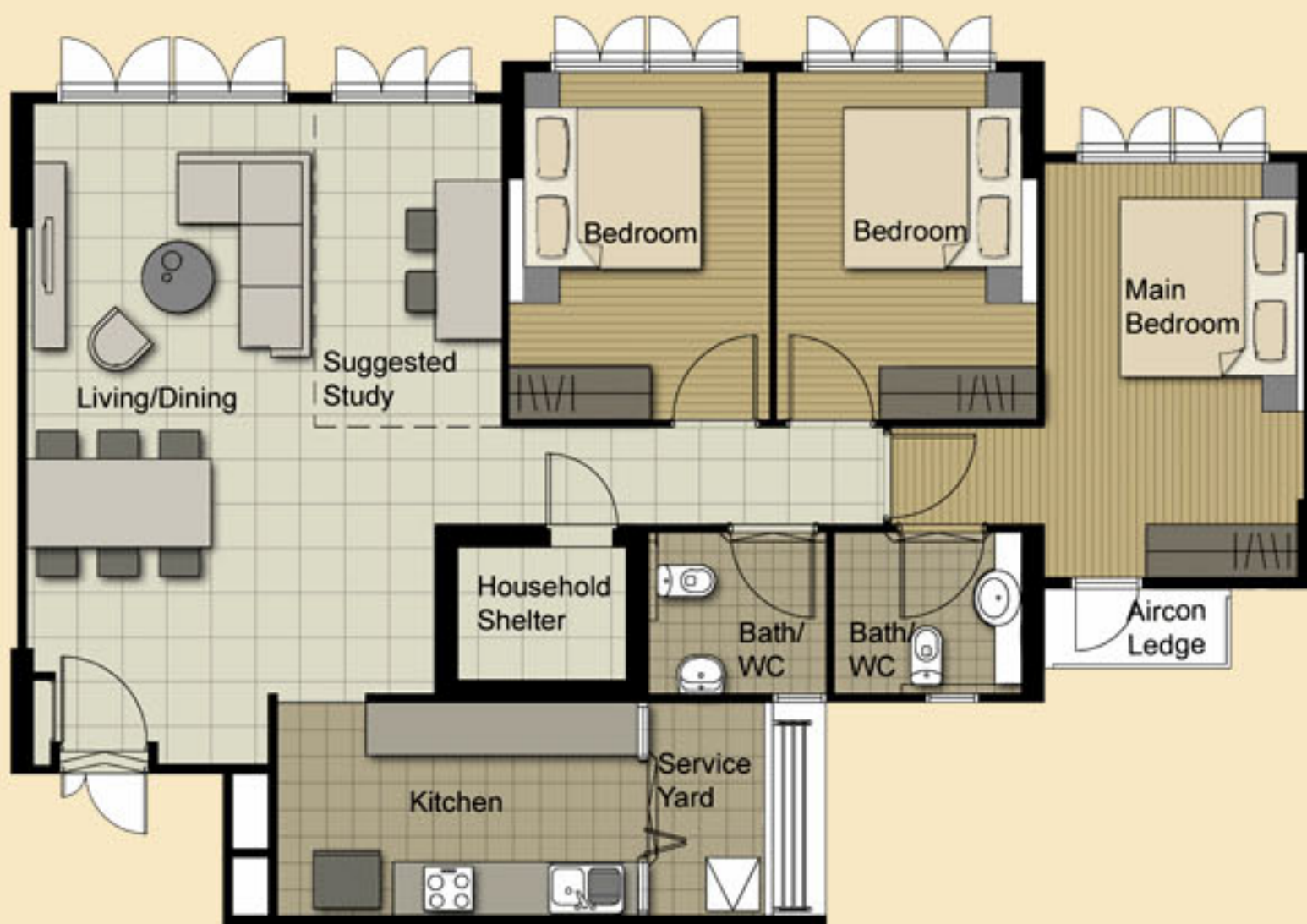
TYPICAL 5-ROOM FLOOR PLAN APPROX. FLOOR AREA 112 sqm (Inclusive of Internal Floor Area 110 sqm and Air-Con Ledge)
