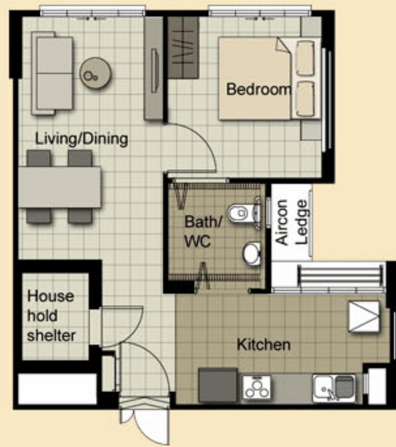
TYPICAL STUDIO APARTMENT (TYPE B) FLOOR PLAN APPROX. FLOOR AREA 46 sqm (Inclusive of Internal Floor Area 45 sqm and Air-Con Ledge)
