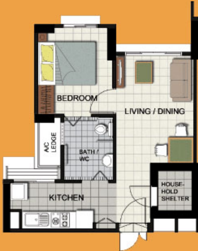
TYPICAL STUDIO APARTMENT (TYPE A) FLOOR PLAN APPROX. FLOOR AREA 37 sqm (Inclusive of Internal Floor Area 35 sqm and Air-Con Ledge)
