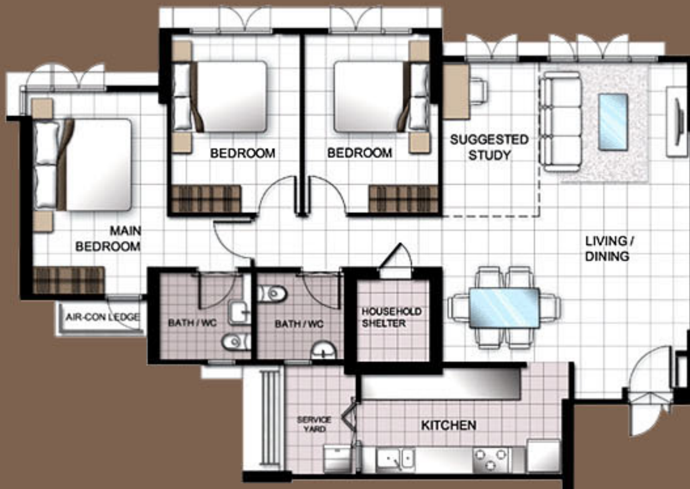
TYPICAL 5-ROOM FLOOR PLAN APPROX. FLOOR AREA 111 sqm (Inclusive of Internal Floor Area 110 sqm and Air-Con Ledge)
