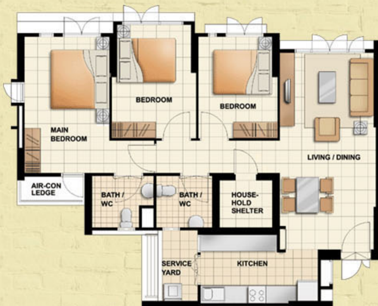
TYPICAL 4-ROOM FLOOR PLAN APPROX. FLOOR AREA 93 sqm (Inclusive of Internal Floor Area 90 sqm and Air-Con Ledge)
