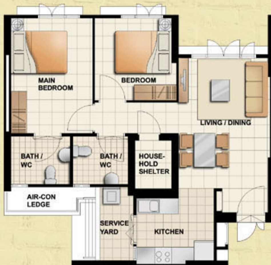
TYPICAL 3-ROOM FLOOR PLAN APPROX. FLOOR AREA 68 sqm (Inclusive of Internal Floor Area 65 sqm and Air-Con Ledge)
