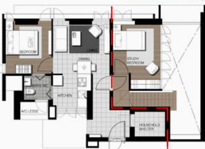
STUDIO APARTMENT FLOOR PLAN APPROX. FLOOR AREA 44 sqm (Inclusive of Internal Floor Area 42 sqm and Air-Con Ledge)
