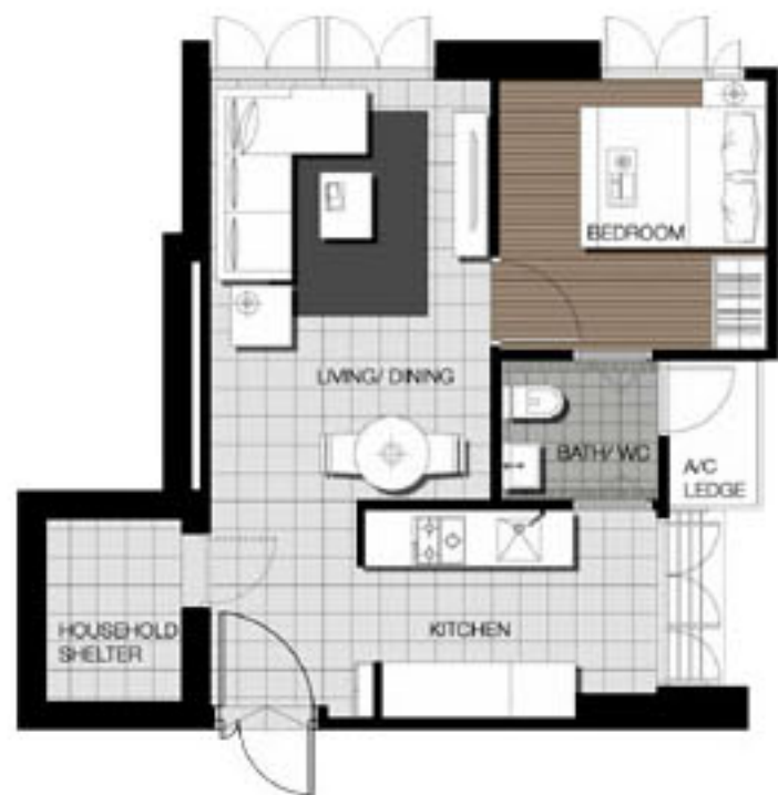
STUDIO APT FLOOR PLAN APPROX. FLOOR AREA 44 sqm (Inclusive of Internal Floor Area 42 sqm and Air-Con Ledge)
