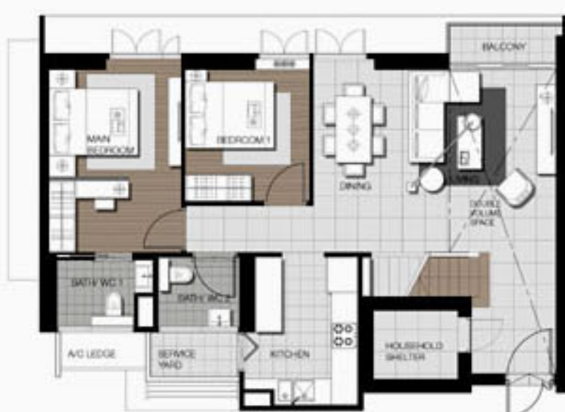
5-ROOM (LOFT 1) LOWER FLOOR PLAN APPROX. FLOOR AREA 122 sqm (Inclusive of Internal Floor Area 103 sqm, Air-Con Ledge and Double Volume Space)
