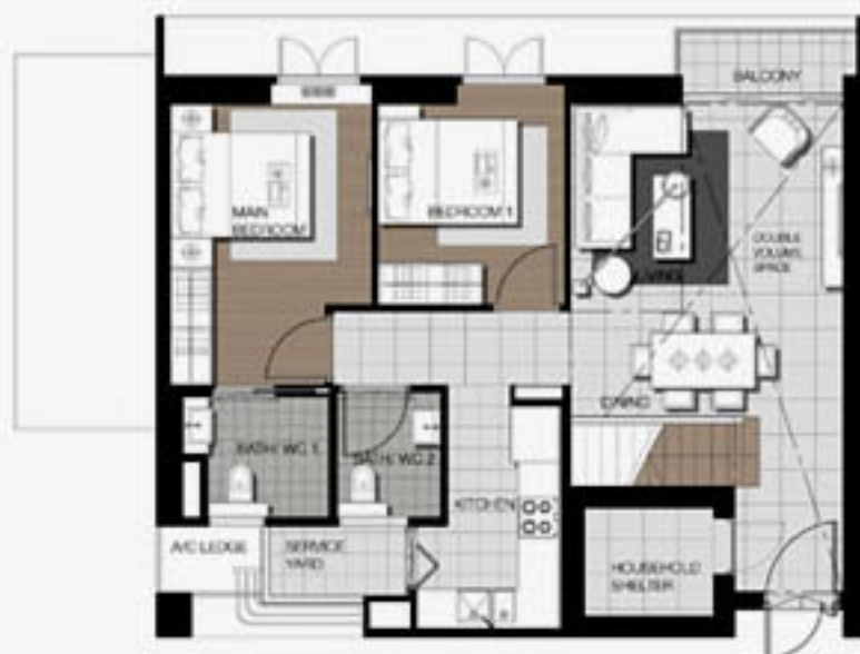
4-ROOM (LOFT 1) LOWER FLOOR PLAN APPROX. FLOOR AREA 109 sqm (Inclusive of Internal Floor Area 88 sqm, Air-Con Ledge and Double Volume Space)
