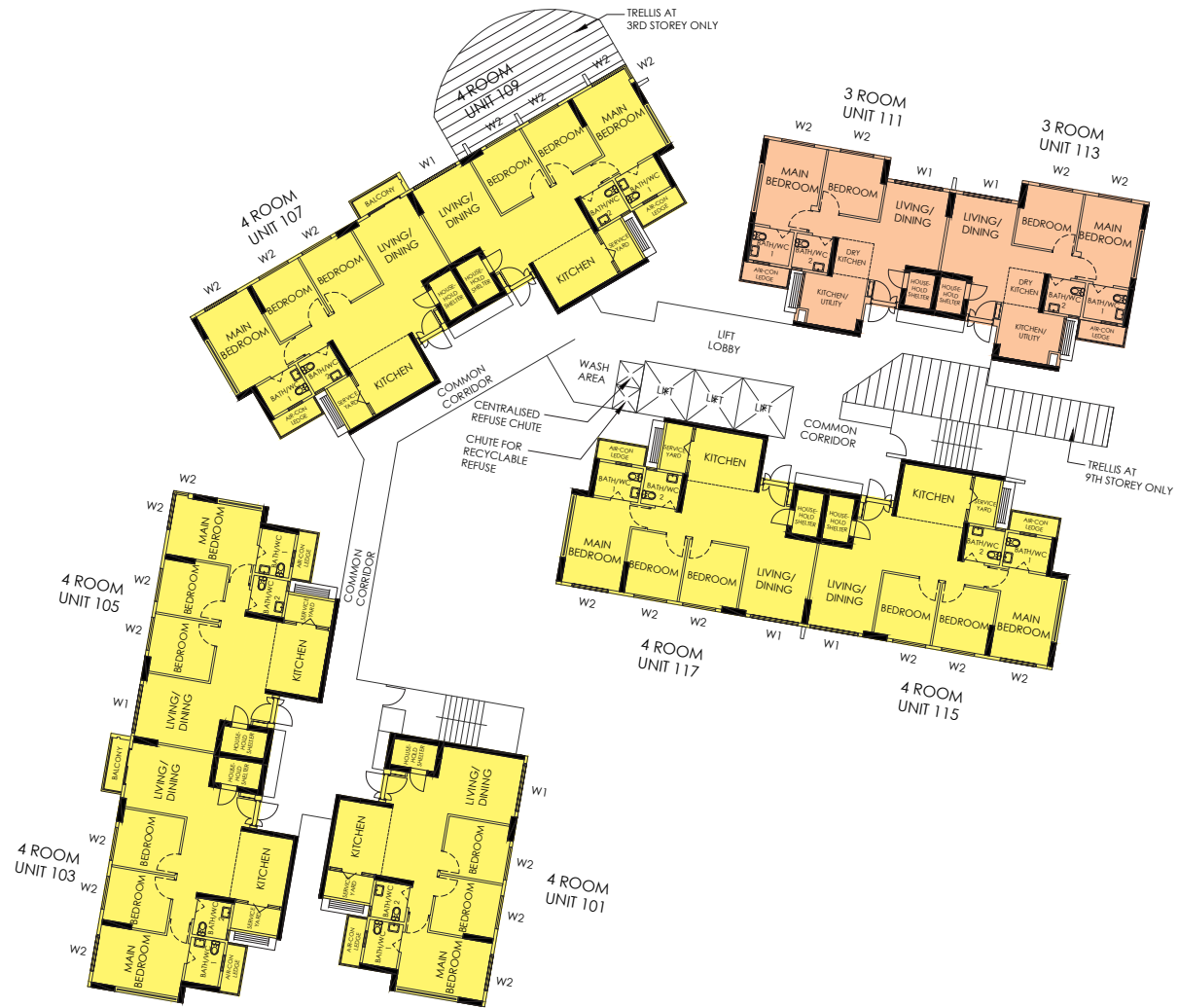
BLOCK 233A (3RD TO 7TH, 9TH TO 12TH STOREY FLOOR PLAN) UNITS AT AND ABOVE 9TH STOREY ARE HIGHER THAN THE MAIN ROOF GARDEN LEVEL OF BLOCK 233
