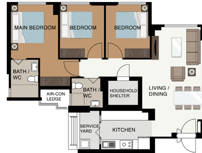
4-ROOM FLOOR PLAN (With Suggested Furniture Layout) APPROX. FLOOR AREA 95 sqm (Inclusive of Internal Floor Area of 92 sqm and Air-Con Ledge)
