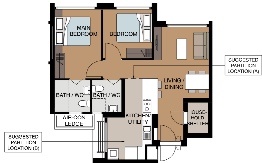
3-ROOM FLOOR PLAN (With Suggested Furniture Layout) APPROX. FLOOR AREA 70 sqm (Inclusive of Internal Floor Area of 68 sqm and Air-Con Ledge)
