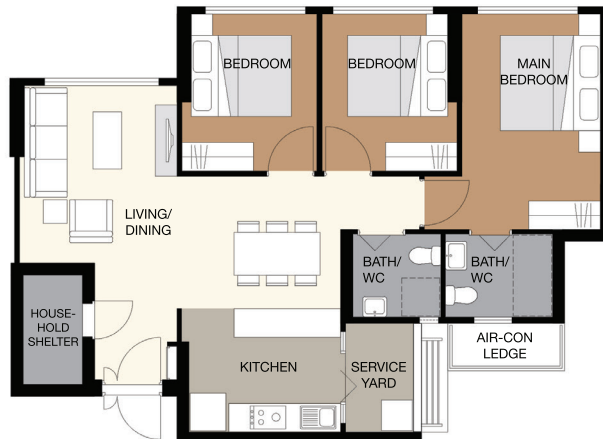
4-ROOM FLOOR PLAN (With Suggested Furniture Layout) APPROX. FLOOR AREA 93 sqm (Inclusive of Internal Floor Area of 90 sqm and Air-con Ledge)
