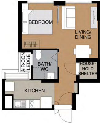
2-ROOM FLEXI (TYPE 1) FLOOR PLAN (With Suggested Furniture Layout) APPROX. FLOOR AREA 38 sqm (Inclusive of Internal Floor Area of 36 sqm and Air-con Ledge)
