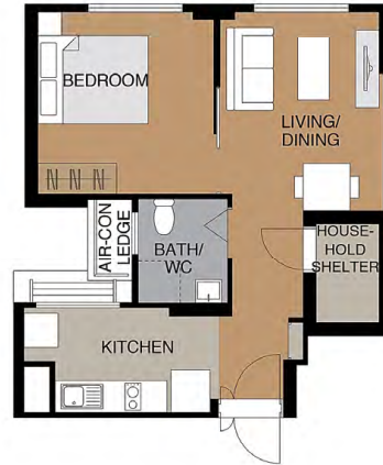
2-ROOM FLEXI (TYPE 2) FLOOR PLAN (With Suggested Furniture Layout) APPROX. FLOOR AREA 47 sqm (Inclusive of Internal Floor Area of 45 sqm and Air-con Ledge)
