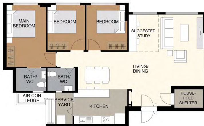
5-ROOM FLOOR PLAN (With Suggested Furniture Layout) APPROX. FLOOR AREA 112 sqm (Inclusive of Internal Floor Area of 110 sqm and Air-con Ledge)
