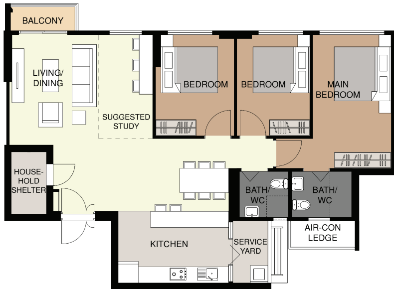
5-ROOM FLOOR PLAN (With Suggested Furniture Layout) APPROX. FLOOR AREA 116 sqm (Inclusive of Internal Floor Area of 113 sqm and Air-Con Ledge)
