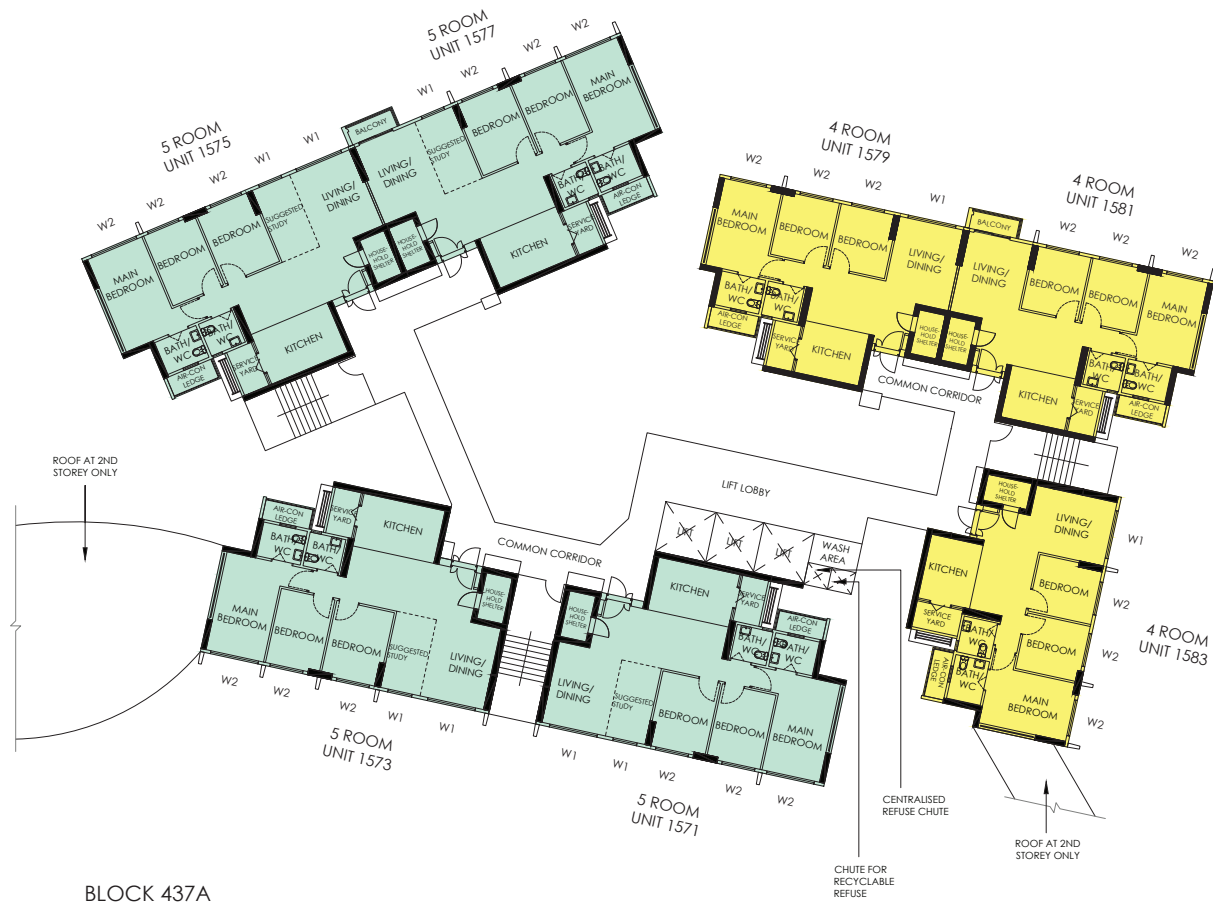
BLOCK 437A (2ND TO 4TH, 6TH TO 12TH STOREY FLOOR PLAN) UNITS AT AND ABOVE 7TH STOREY ARE HIGHER THAN THE MAIN ROOF GARDEN LEVEL OF BLOCK 435
