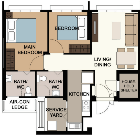
LAYOUT IDEAS FOR 3-ROOM APPROX. FLOOR AREA 68 sqm (Inclusive of Internal Floor Area of 65 sqm and Air-Con Ledge)
