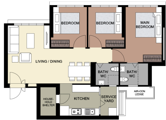
LAYOUT IDEAS FOR 4-ROOM APPROX. FLOOR AREA 93 sqm (Inclusive of Internal Floor Area of 90 sqm and Air-Con Ledge)
