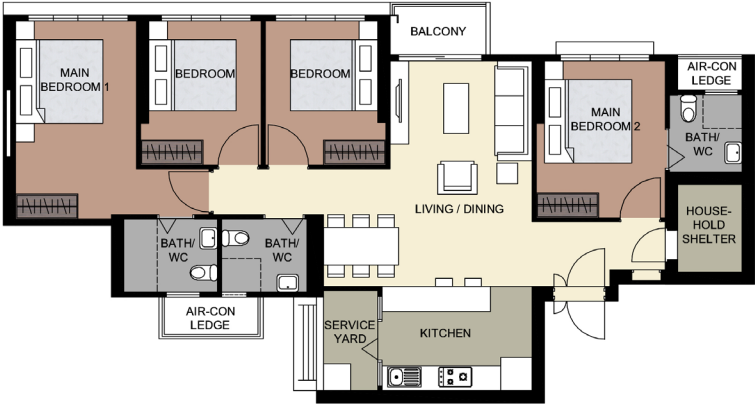
LAYOUT IDEAS FOR 3GEN FLAT APPROX. FLOOR AREA 123 sqm (Inclusive of Internal Floor Area of 118 sqm and Air-Con Ledges)
