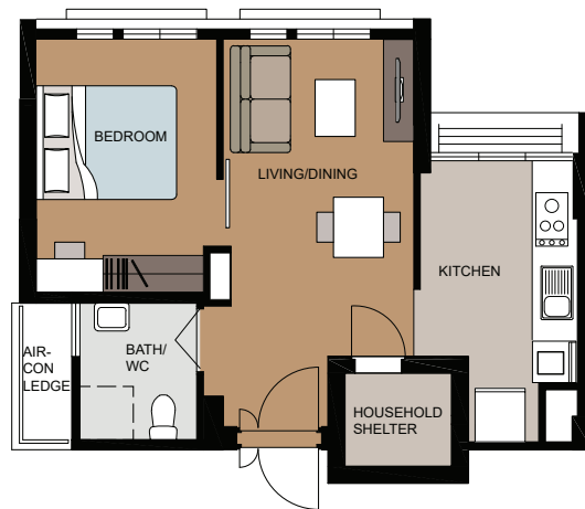
LAYOUT IDEAS FOR 2 ROOM FLEXI (TYPE 2) APPROX. FLOOR AREA 47 sqm (Inclusive of Internal Floor Area of 45 sqm and Air-Con Ledge)
