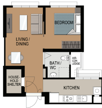
LAYOUT IDEAS FOR 2-ROOM FLEXI (TYPE 2) APPROX. FLOOR AREA 47 sqm (Inclusive of Internal Floor Area of 45 sqm and Air-Con Ledge)
