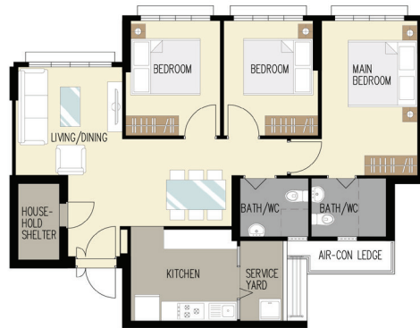
TYPICAL 4-ROOM FLOOR PLAN APPROX. FLOOR AREA 94 sqm ( Inclusive of Internal Floor Area of 90 sqm and Air-Con Ledge )
