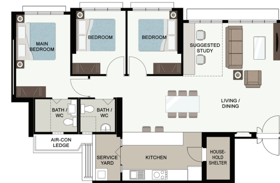
LAYOUT IDEAS FOR 5-ROOM APPROX. FLOOR AREA 113 sqm (Inclusive of Internal Floor Area of 110 sqm and Air-con Ledge)
