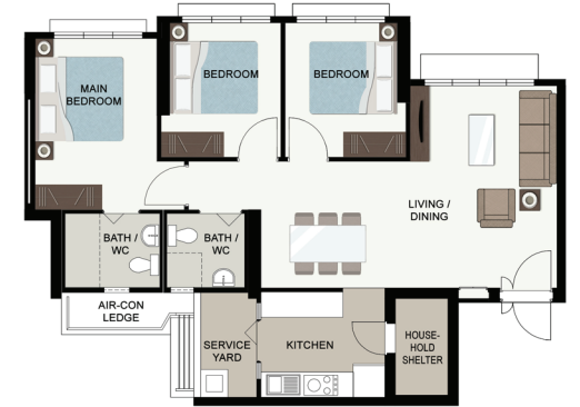
LAYOUT IDEAS FOR 4-ROOM APPROX. FLOOR AREA 93 sqm (Inclusive of Internal Floor Area of 90 sqm and Air-con Ledge)
