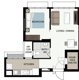
LAYOUT IDEAS FOR 2-ROOM FLEXI (TYPE 2) APPROX. FLOOR AREA 47 sqm (Inclusive of Internal Floor Area of 45 sqm and Air-con Ledge)
