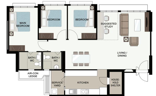
LAYOUT IDEAS FOR 5-ROOM APPROX. FLOOR AREA 113 sqm (Inclusive of Internal Floor Area of 110 sqm and Air-con Ledge)
