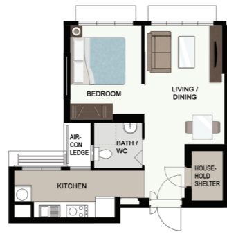
LAYOUT IDEAS FOR 2-ROOM FLEXI (TYPE 2) APPROX. FLOOR AREA 47 sqm (Inclusive of Internal Floor Area 45 sqm and Air-Con Ledge)
