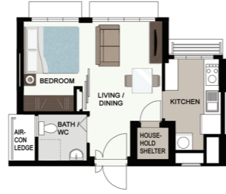
LAYOUT IDEAS FOR 2-ROOM FLEXI (TYPE 1) APPROX. FLOOR AREA 38 sqm (Inclusive of Internal Floor Area 36 sqm and Air-Con Ledge)
