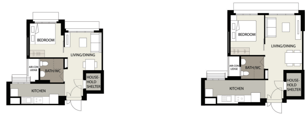
LAYOUT IDEAS FOR 2-ROOM FLEXI (TYPE 1) APPROX. FLOOR AREA 38 sqm (Inclusive Of Internal Floor Area 36 sqm and Air-Con Ledge)
