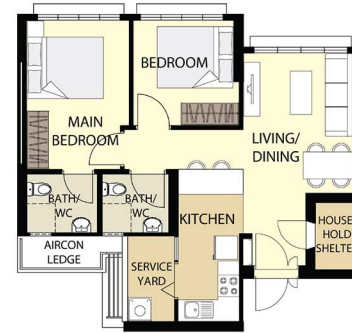
LAYOUT IDEAS FOR 3 ROOM Approx. Floor Area of 68 sqm (Inclusive of Internal Floor Area of 65 sqm and Aircon Ledge)
