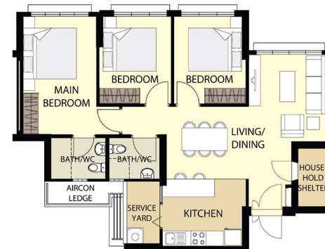
LAYOUT IDEAS FOR 4 ROOM Approx. Floor Area of 94 sqm (Inclusive of Internal Floor Area of 90 sqm and Aircon Ledge)
