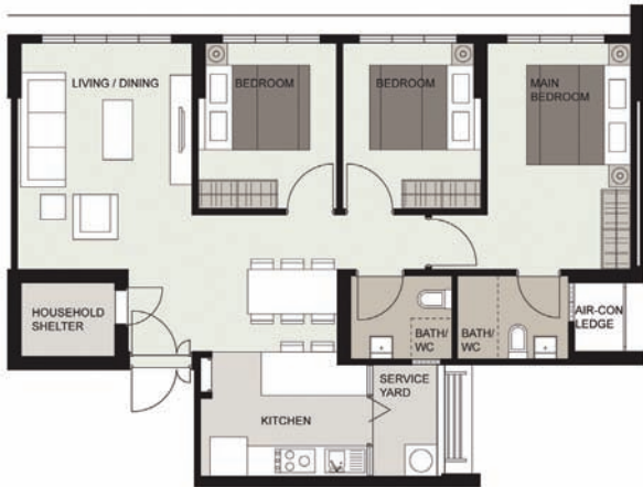
LAYOUT IDEAS FOR 4-ROOM APPROX. FLOOR AREA 92 sqm (Inclusive of Internal Floor Area of 90 sqm and Air-Con Ledge)
