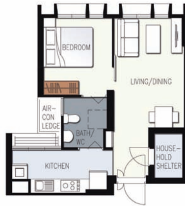
LAYOUT IDEAS FOR 2-ROOM (TYPE 2) APPROX. FLOOR AREA OF 47 sqm (Inclusive of Internal Floor Area of 45 sqm and Air-Con Ledge)
