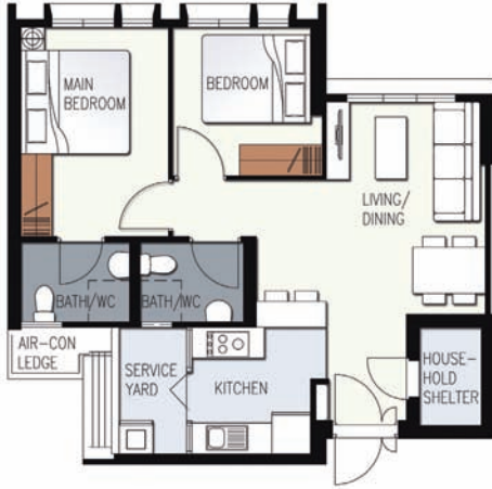
LAYOUT IDEAS FOR 3-ROOM APPROX. FLOOR AREA OF 67 sqm (Inclusive of Internal Floor Area of 65 sqm and Air-Con Ledge)
