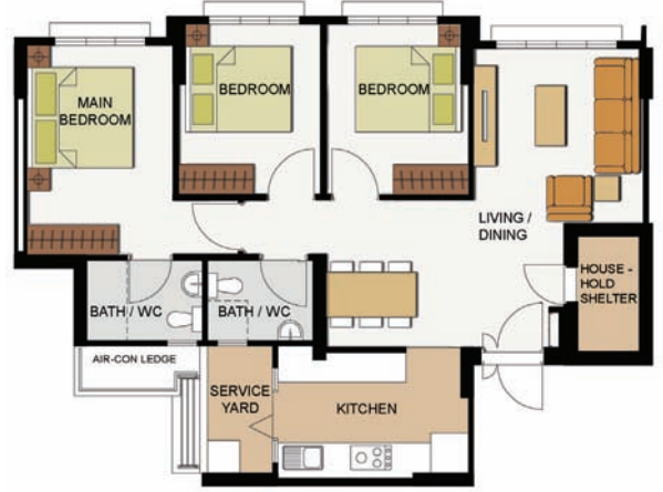
With Kitchen Partition Wall
