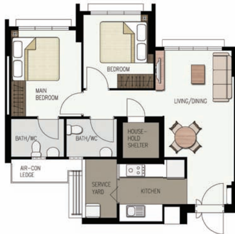
LAYOUT IDEAS FOR 3-ROOM APPROX. FLOOR AREA 68 sqm (Inclusive of Internal Floor Area of 65 sqm and Air-Con Ledge)
