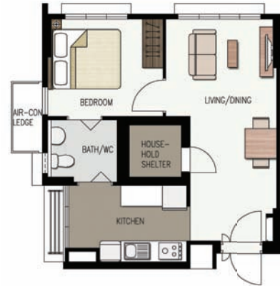
LAYOUT IDEAS FOR 2-ROOM (TYPE 2) APPROX. FLOOR AREA 47 sqm (Inclusive of Internal Floor Area of 45 sqm and Air-Con Ledge)
